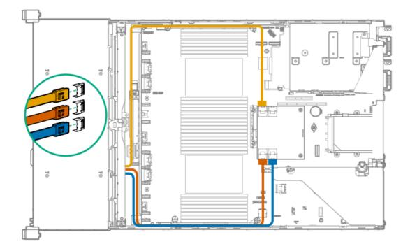
Cable routing: System board processor 1 (ports 1A and 2A) to slotted expansion board ports 1-2 in the primary riser
