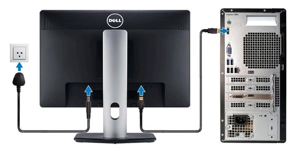
(i) **NOTE:** If you ordered your computer with a discrete graphics card, the HDMI and VGA ports on the back panel of your computer are covered. Connect the display to the discrete graphics card.
