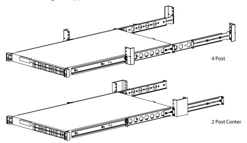
Note: When tightening the loose rails, support the bottom of the server to ensure proper rail adjustment
