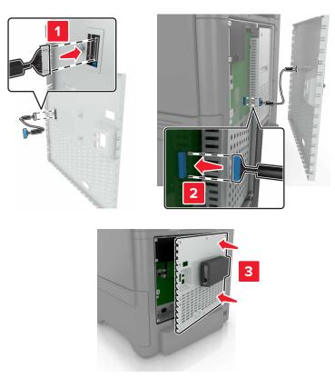
7 Reattach the controller board access cover.
