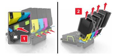
**5** Unpack the new imaging kit, and then remove the packing material.
