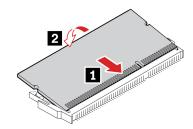
**Note:** During the installation, ensure that you align the memory module to the slot and press down on both ends until the latches are fully engaged with a click.
