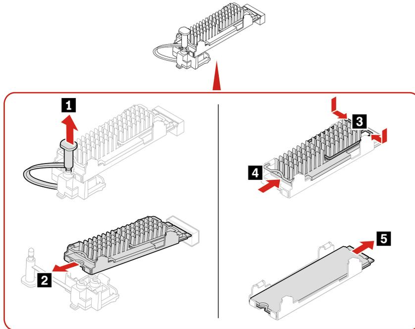
**Note:** Remove the film that covers the thermal pad (if any) when installing the M.2 solid-state drive and the heat sink.
