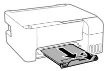
4. If you are inserting a stack of paper, fan the sheets first and tap the stack on a flat surface to even the edges.
