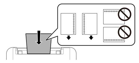
• To load a sheet of paper longer than legal size, close the paper support and flatten the leading edge of the paper as shown.
