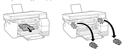
**Caution:** When removing jammed paper, avoid tilting the printer, placing it vertically, or turning it upside down; otherwise ink may leak.
