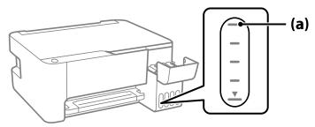
5. Position the top of the ink bottle along the slot in front of the filling port, then slowly stand the bottle up to insert it. Wait for the ink to fill the tank. Do not squeeze the bottle. Ink flows into the tank and stops automatically when the ink is filled to the upper line.
