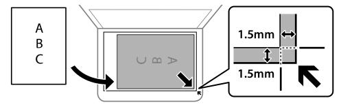
**Note:** You can place multiple originals on the scanner glass. Just make sure they are at least 0.2 inch (4.5 mm) away from the edge of the scanner glass and at least 0.8 inch (20 mm) away from each other.
