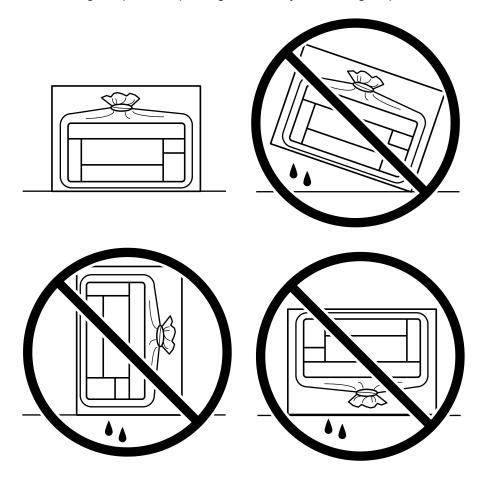
When storing or transporting an ink bottle after removing its seal, do not tilt the bottle and do not subject it to impacts or temperature changes. Otherwise, ink may leak even if the cap on the ink bottle is tightened securely. Be sure to keep the ink bottle upright when tightening the cap, and take measures to prevent ink from leaking when transporting the ink bottles. • Do not put opened ink bottles in the box with the product.
