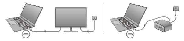
In another scenario, if you carry your computer around without the included ac power adapter, you may use a capable USB-C charger to provide power through the right USB-C port. In both scenarios, the output power of a USB-C charger or the USB-C port on a dock or display should be at least 20 V and 2.25 A in order to provide power to your computer. The following table lists the charging capability of a USB-C port on a charger or an external device based on its maximum output power.
