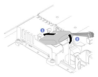
Figure 66. Flash power module installation
