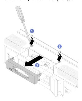
Figure 132. VGA cable removal
