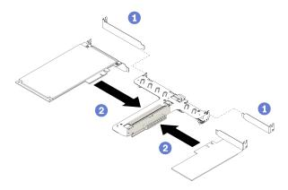
Figure 41. Adapter installation
