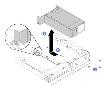
Figure 91. Power supply unit removal
