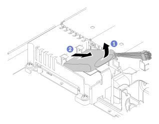
Figure 65. Flash power module removal
