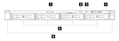
Figure 6. Four hot-swap drives model front view
