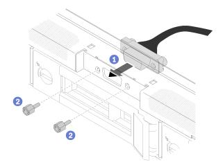
Figure 134. VGA cable installation
