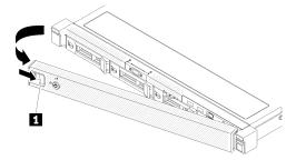
Figure 118. Security bezel removal
