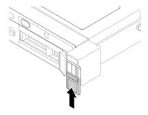
Figure 114. ID label installation
