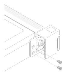
Figure 113. Rack latches installation
