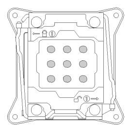
Figure 106. Proper shape of the thermal grease
