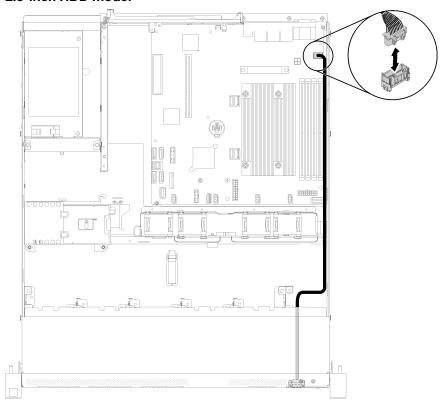
Figure 25. Front VGA cable routing with ten drives
