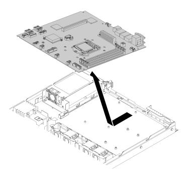
Figure 122. System board removal
