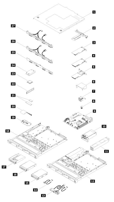
Figure 39. Server components - 3.5-inch drive model
