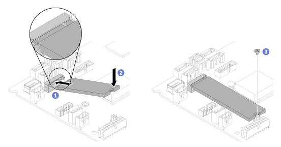
Figure 85. M.2 drive installation
