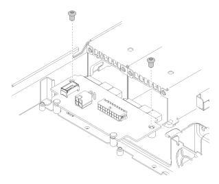
Figure 98. Power interface board screw removal
