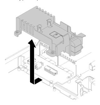
Figure 97. Power interface board cover removal
