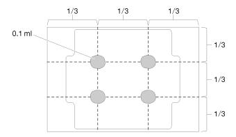
Figure 105. Proper shape of the thermal grease
