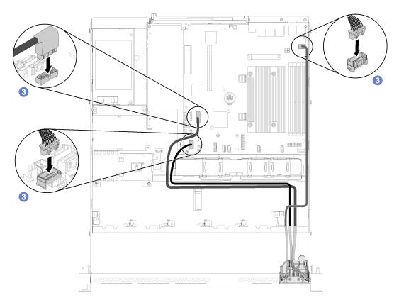
Figure 72. Front operator panel (2.5-inch HDD model) cable routing
