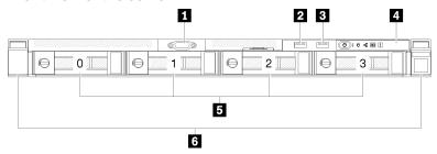
Figure 5. Four simple-swap drives model front view
