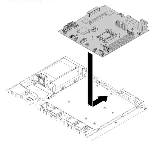
Figure 123. System board installation
