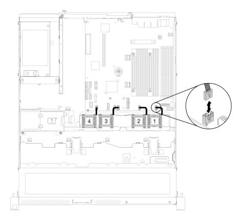
Figure 26. Fan cable routing
