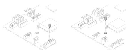
Figure 84. Hex screw location for 80 mm/42 mm M.2 drive
