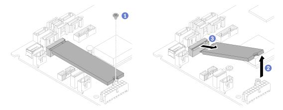
Figure 82. M.2 drive removal
