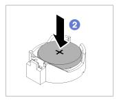
Figure 51. CMOS battery installation
