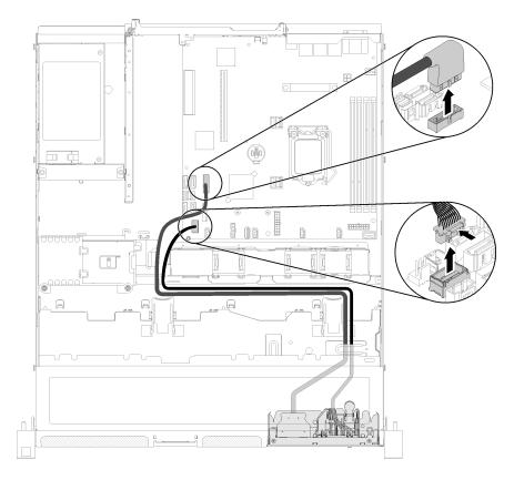
Figure 73. Front operator panel (3.5-inch HDD model) removal
