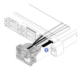
Figure 70. Front operator panel (2.5-inch HDD model) installation
