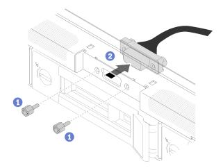
Figure 133. VGA cable removal
