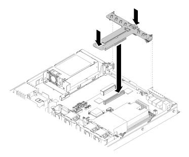
Figure 90. PCIe riser assembly installation
