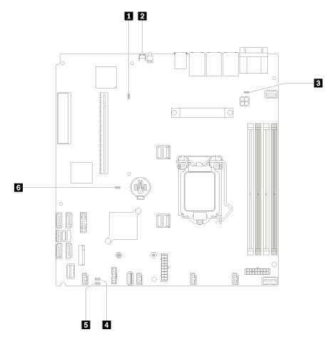
Figure 15. System-board jumpers and buttons
