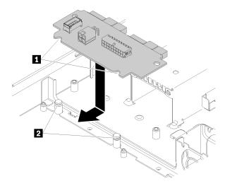
Figure 100. Power interface board installation
