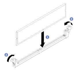
Figure 55. DIMM installation
