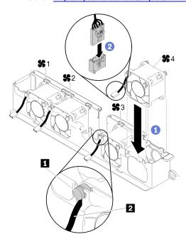
Figure 63. Fan installation
