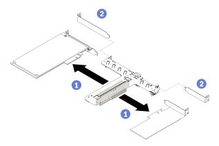
Figure 40. Adapter removal
