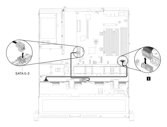
Figure 32. Four 3.5-inch hot-swap drive model with software RAID
