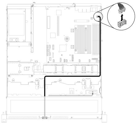
Figure 24. Front VGA cable routing with four drives
