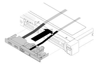
Figure 76. Front operator panel (3.5-inch HDD model) installation
