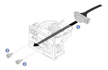
Figure 130. VGA cable installation
