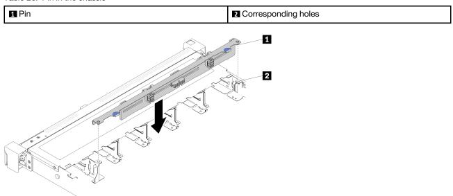
Figure 47. 3.5-inch hot-swap drive backplane installation
