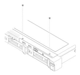
Figure 74. Front operator panel removal
