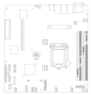
Figure 52. DIMM connectors
