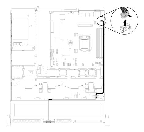
Figure 131. VGA cable removal - 3.5-inch HDD model
