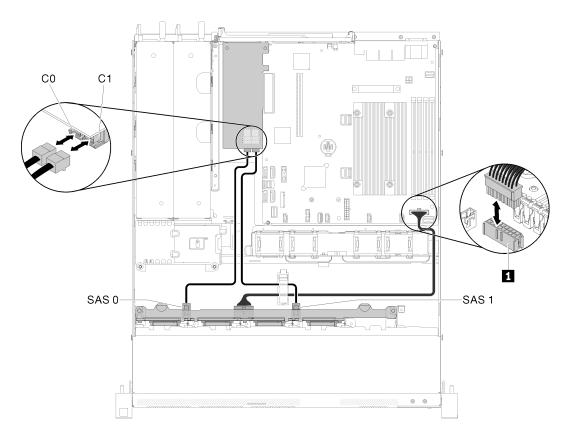
Figure 35. Eight 2.5-inch hot-swap drive model with hardware RAID
