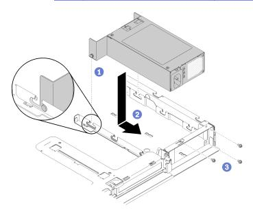
Figure 92. Power supply unit installation
