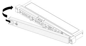
Figure 119. Security bezel installation
