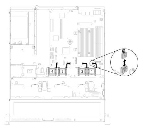
Figure 64. Fan power cable routing
