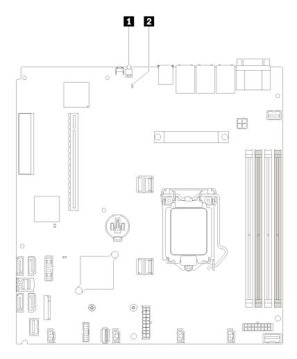
Figure 13. System-board LEDs
