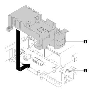
Figure 102. Power interface board cover installation
