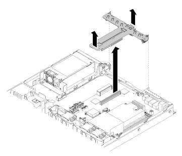
Figure 86. PCIe riser assembly removal
