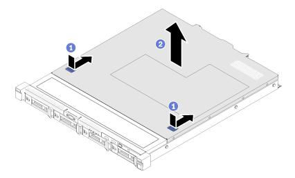
Figure 125. Top cover removal
