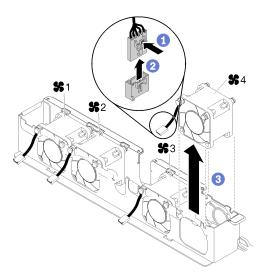
Figure 62. Fan removal
