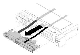
Figure 75. Front operator panel removal
