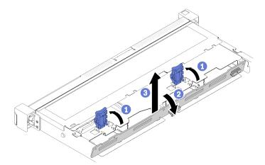
Figure 48. Backplate removal
