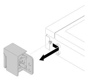
Figure 111. Rack latches removal
