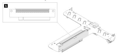
Figure 22. x16 PCIe riser assembly
