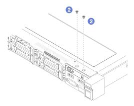
Figure 71. Screws installation
