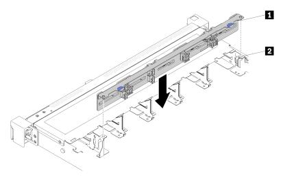
Figure 46. 2.5-inch hot-swap drive backplane installation
