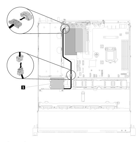
Figure 29. Flash power module cable routing
