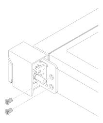
Figure 110. Rack latches removal
