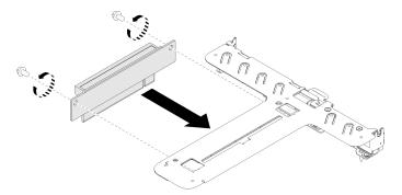
Figure 88. PCIe riser card installation
