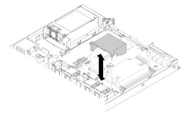
Figure 42. Air baffle removal
