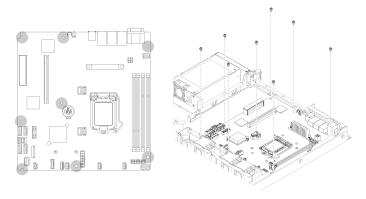
Figure 124. System-board screws location
