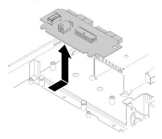
Figure 99. Power interface board removal
