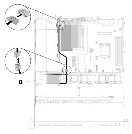
Figure 95. Disconnecting the flash power module cable
