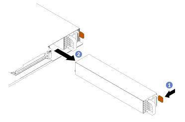
Step 1. Press the release tab toward the handle and carefully pull the handle at the same time to slide the hot-swap power supply unit out of the chassis.
