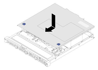
Figure 126. Top cover installation
