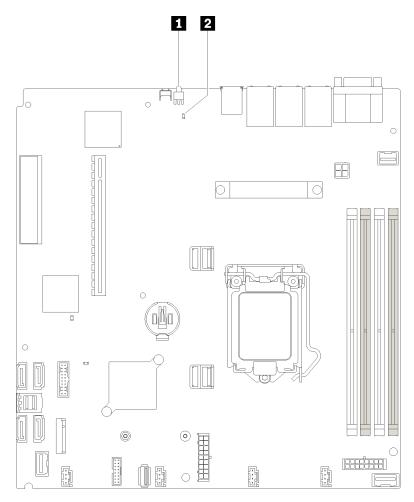
Figure 143. System-board LEDs
