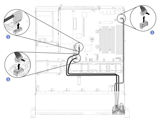
Figure 67. Front operator panel (2.5-inch HDD model) cables removal
