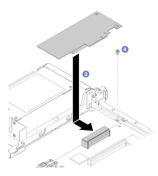
Figure 116. RAID adapter installation
