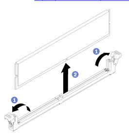
Figure 53. DIMM removal
