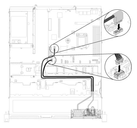
Figure 78. Front operator panel installation
