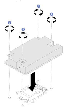
Figure 80. Heat sink installation
