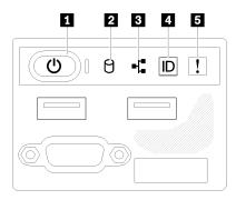
Figure 9. 2.5-inch drive chassis front I/O assembly
