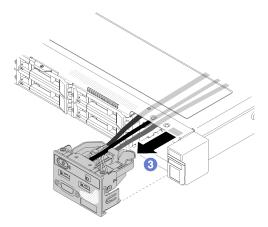
Figure 69. Front operator panel removal
