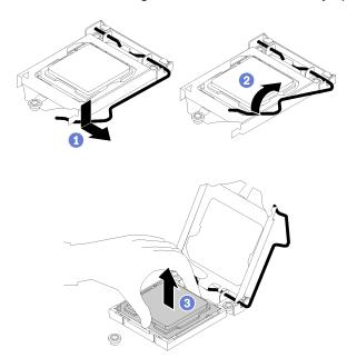
Figure 104. Opening the processor retainer
