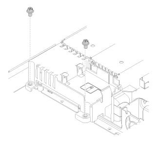
Figure 96. Cover screw removal
