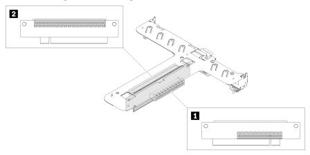
Figure 23. x8/x8 Butterfly riser assembly
