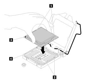
Figure 107. Installing the processor
