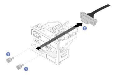
Figure 129. VGA cable removal - 2.5-inch HDD model
