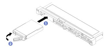
Figure 57. Simple-swap drive installation
