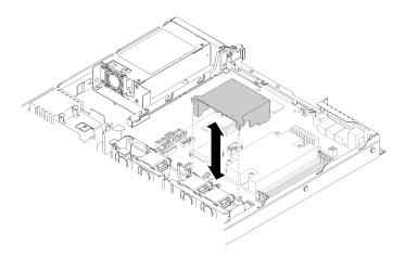
Figure 43. Air baffle installation
