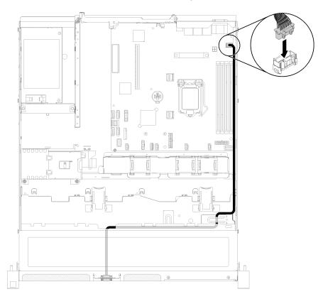
Figure 135. VGA cable installation
