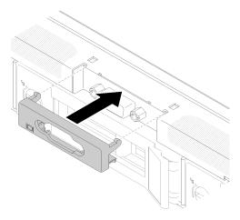
Figure 136. VGA cable installation
