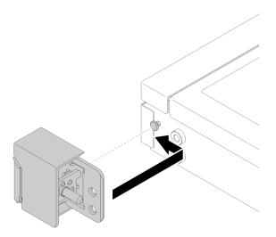
Figure 112. Rack latches installation
