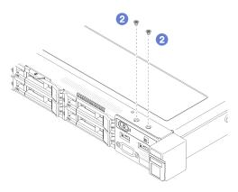
Figure 68. Screws removal
