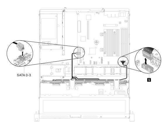
Figure 30. 3.5-inch simple-swap drive model with software RAID
