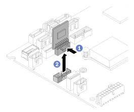
Figure 127. TPM card (for China only) removal
