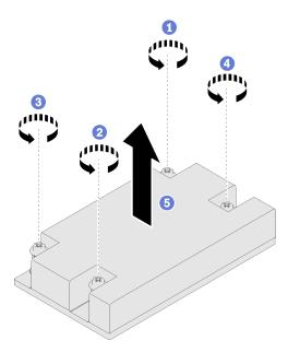
Figure 79. Heat sink removal
