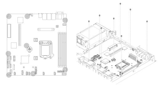
Figure 121. System-board screws location
