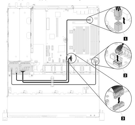
Figure 28. Hot-swap power supply unit cable routing
