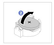
Figure 50. CMOS battery removal
