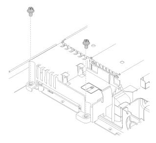
Figure 103. Cover screw installation
