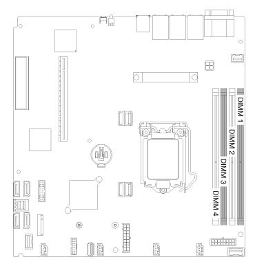
Figure 54. DIMM connectors
