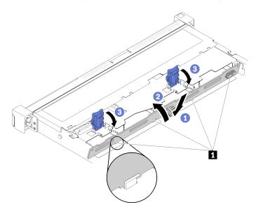
Figure 49. Backplate installation
