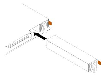
Figure 94. Hot-swap power supply unit installation
