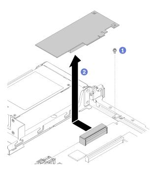
Figure 115. RAID adapter removal
