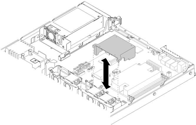
Figure 42. Air baffle removal
