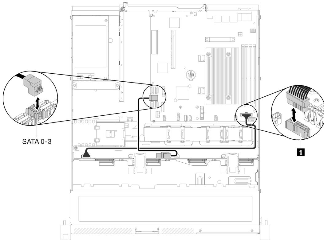
Figure 32. Four 3.5-inch hot-swap drive model with software RAID
