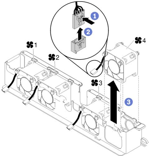
Figure 62. Fan removal
