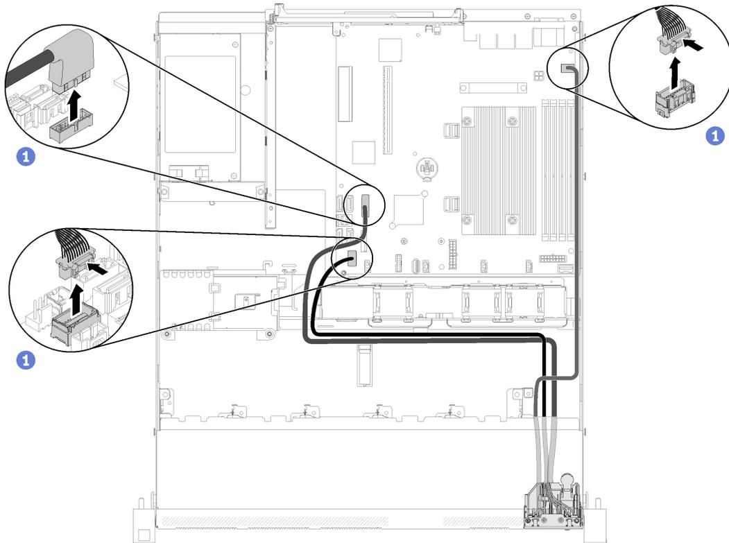
Figure 67. Front operator panel (2.5-inch HDD model) cables removal
