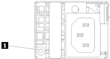
Figure 142. 450 watts Power supply LED
