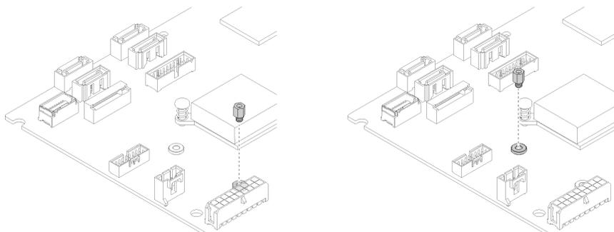
Figure 84. Hex screw location for 80 mm/42 mm M.2 drive
