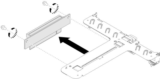
Figure 87. PCIe riser card removal
