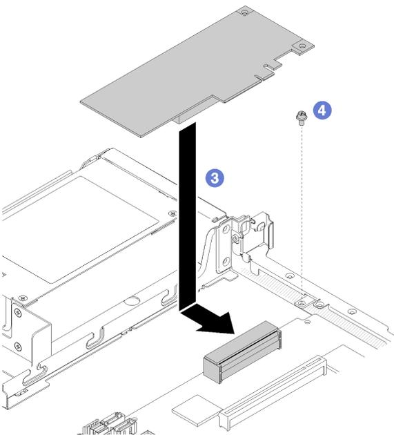
Figure 116. RAID adapter installation
