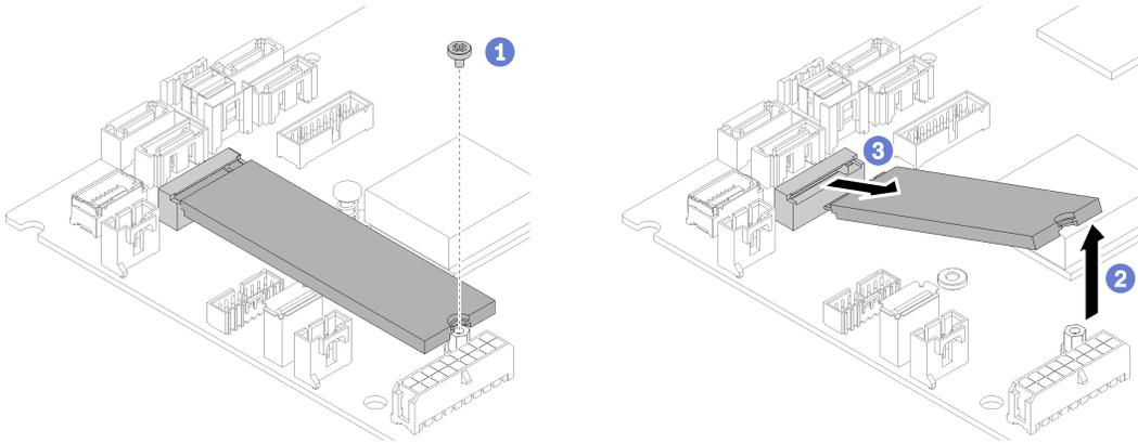
Figure 82. M.2 drive removal
