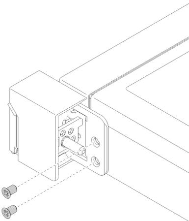
*Figure 110. Rack latches removal*
