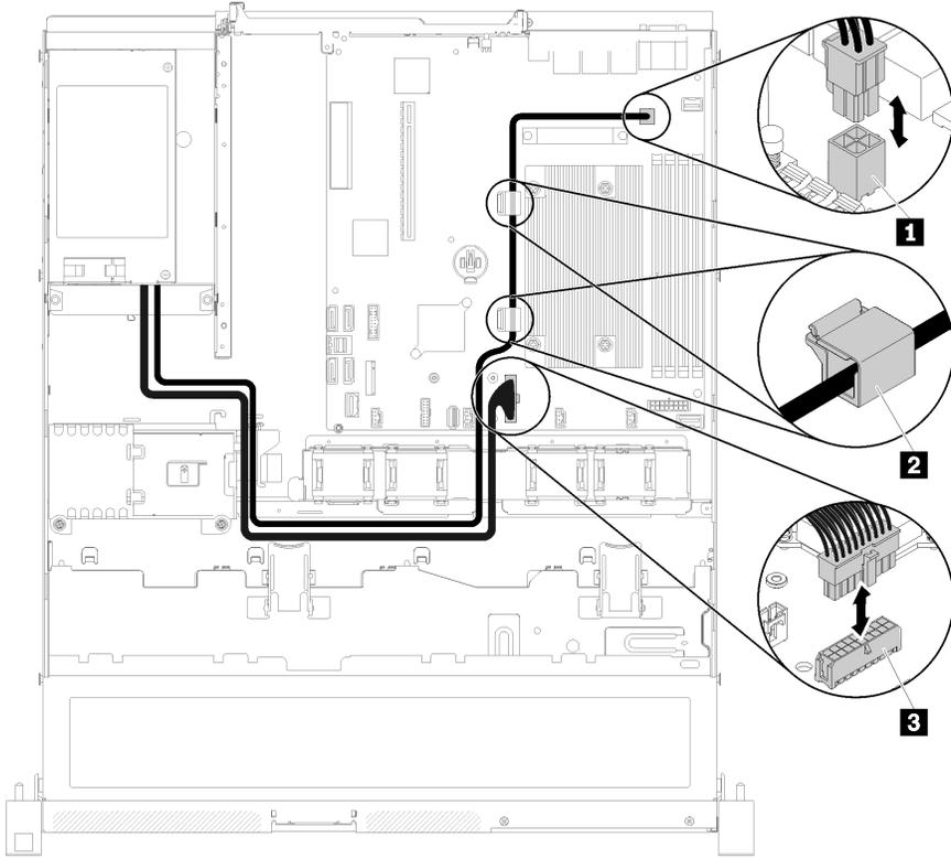
Figure 27. Fixed power supply unit cable routing
