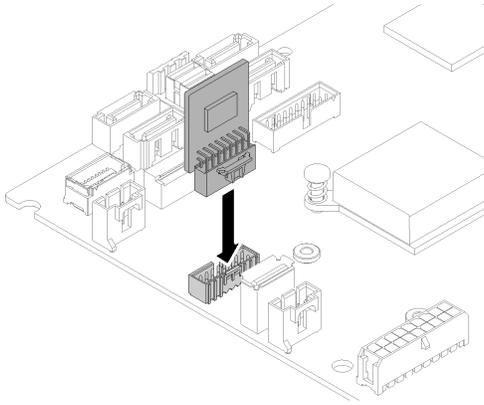
Figure 128. TPM card (for China only) installation
