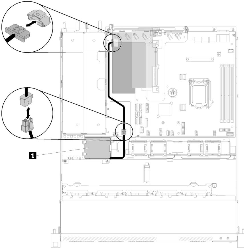
Figure 29. Flash power module cable routing
