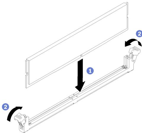
Figure 55. DIMM installation
