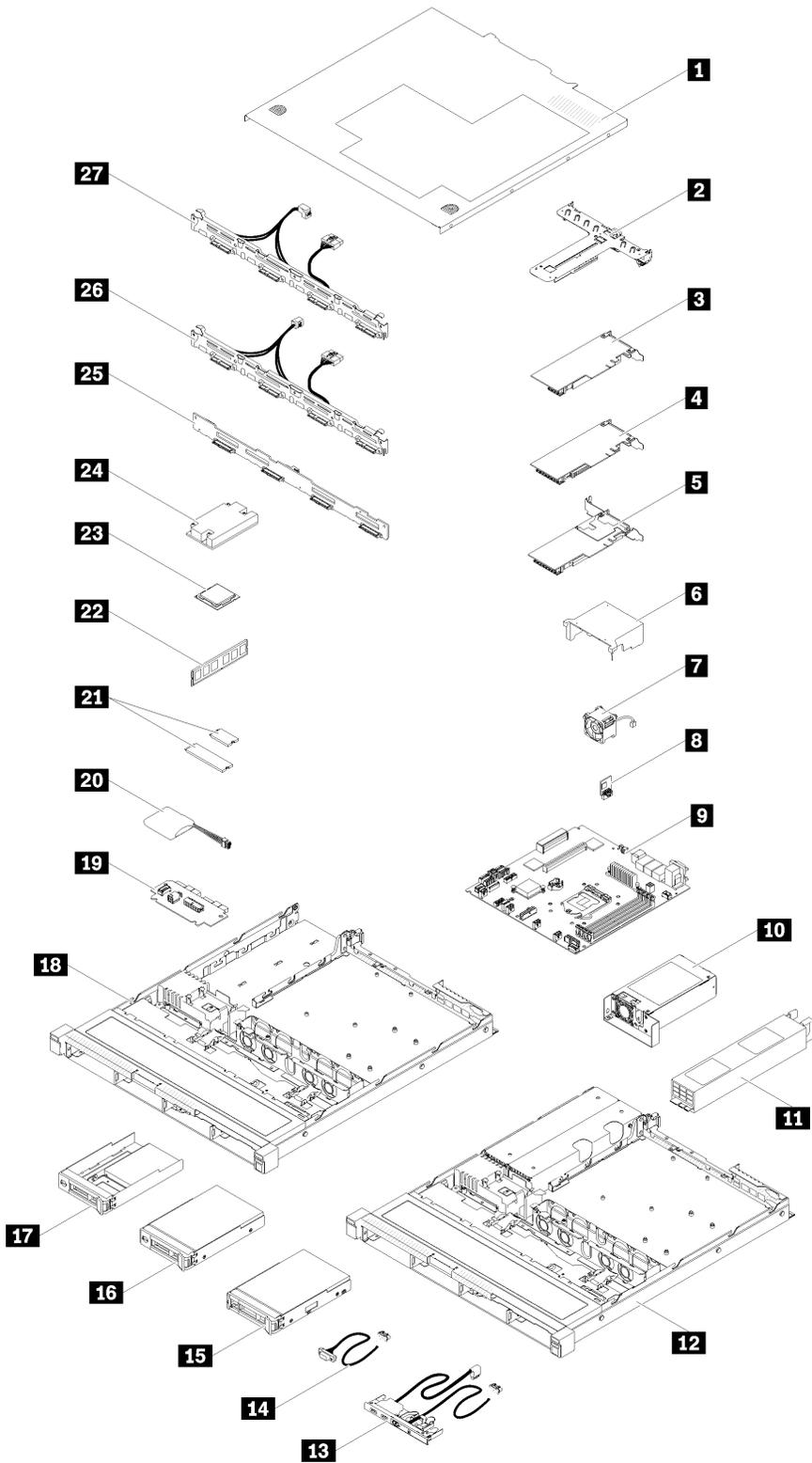
Figure 39. Server components - 3.5-inch drive model
