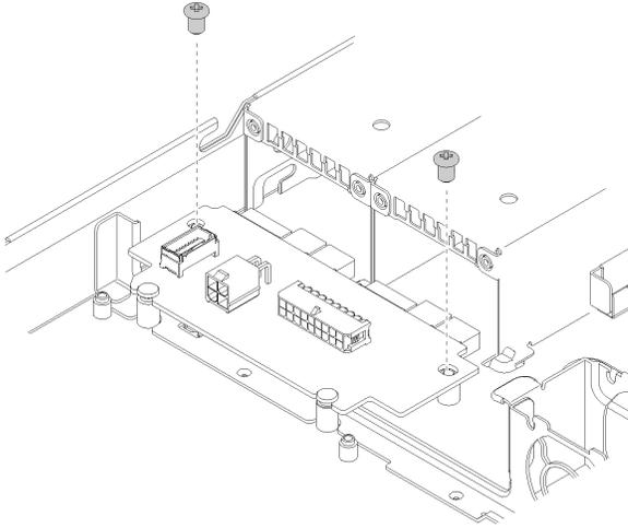
Figure 98. Power interface board screw removal
