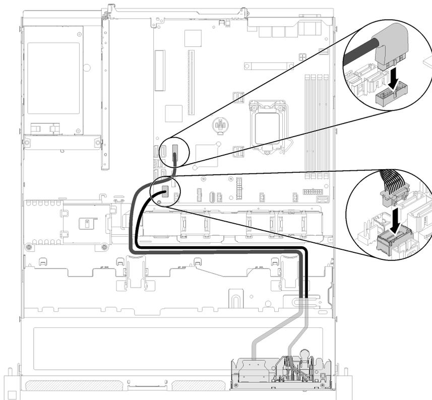
Figure 78. Front operator panel installation
