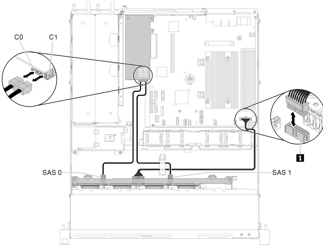
Figure 35. Eight 2.5-inch hot-swap drive model with hardware RAID
