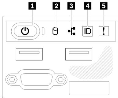
Figure 139. 2.5-inch drive chassis front operator panel
