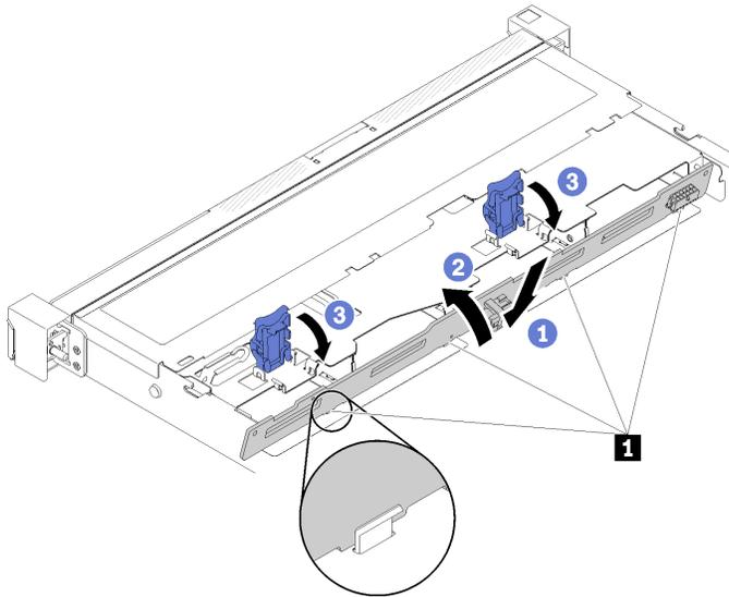
Figure 49. Backplate installation
