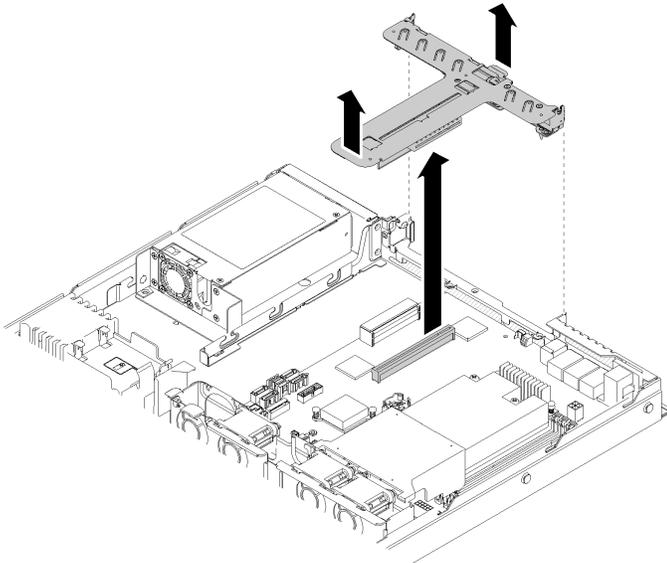
Figure 86. PCIe riser assembly removal
