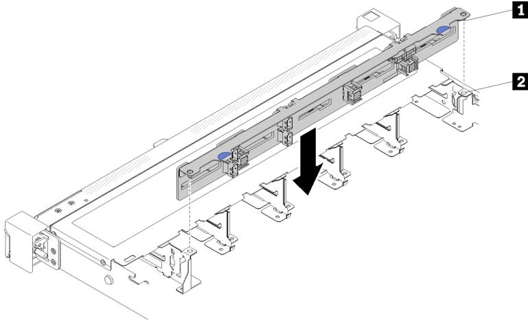
Figure 46. 2.5-inch hot-swap drive backplane installation
