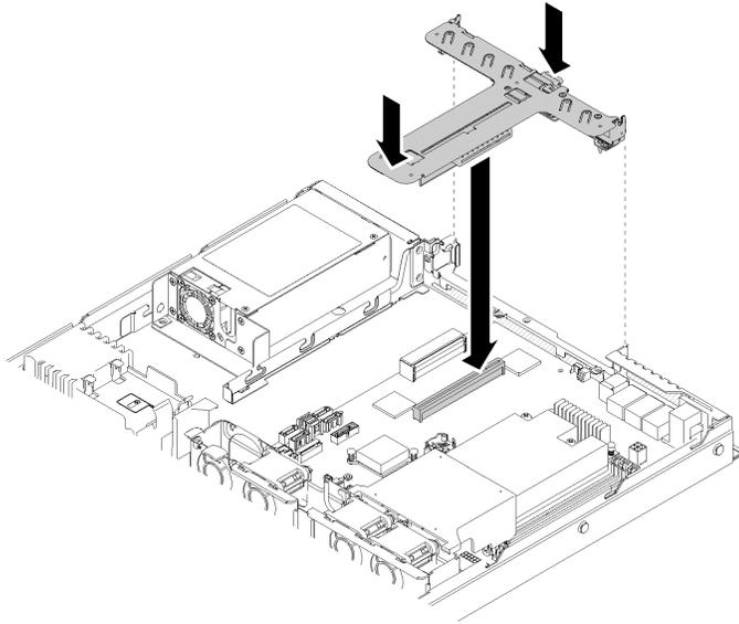
Figure 90. PCIe riser assembly installation
