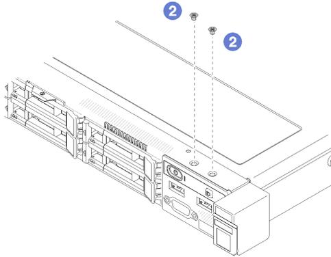
Figure 71. Screws installation
