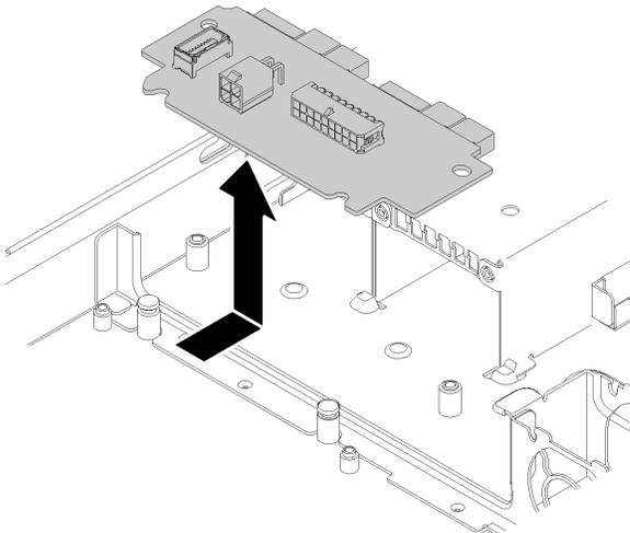
Figure 99. Power interface board removal
