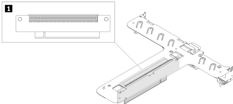
Figure 22. x16 PCIe riser assembly
