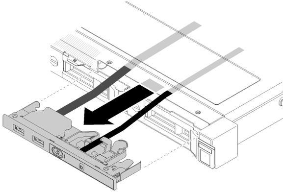
Figure 75. Front operator panel removal
