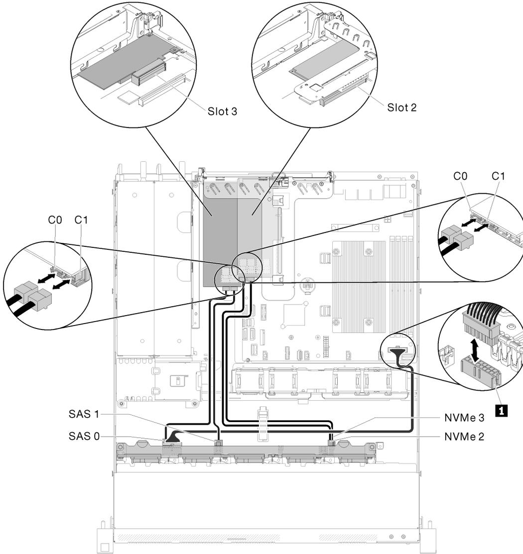
Figure 37. Ten 2.5-inch hot-swap drive model (two NVMe drives supported)
