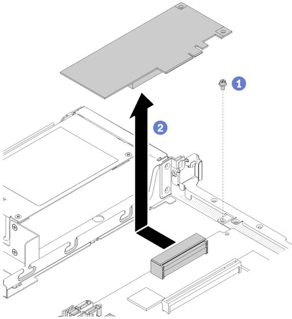
Figure 115. RAID adapter removal
