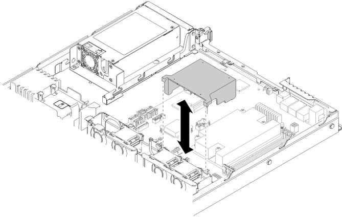
Figure 43. Air baffle installation
