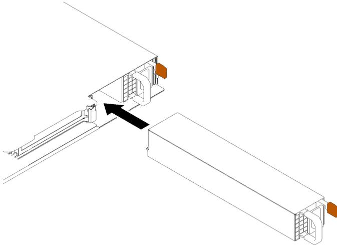
Figure 94. Hot-swap power supply unit installation
