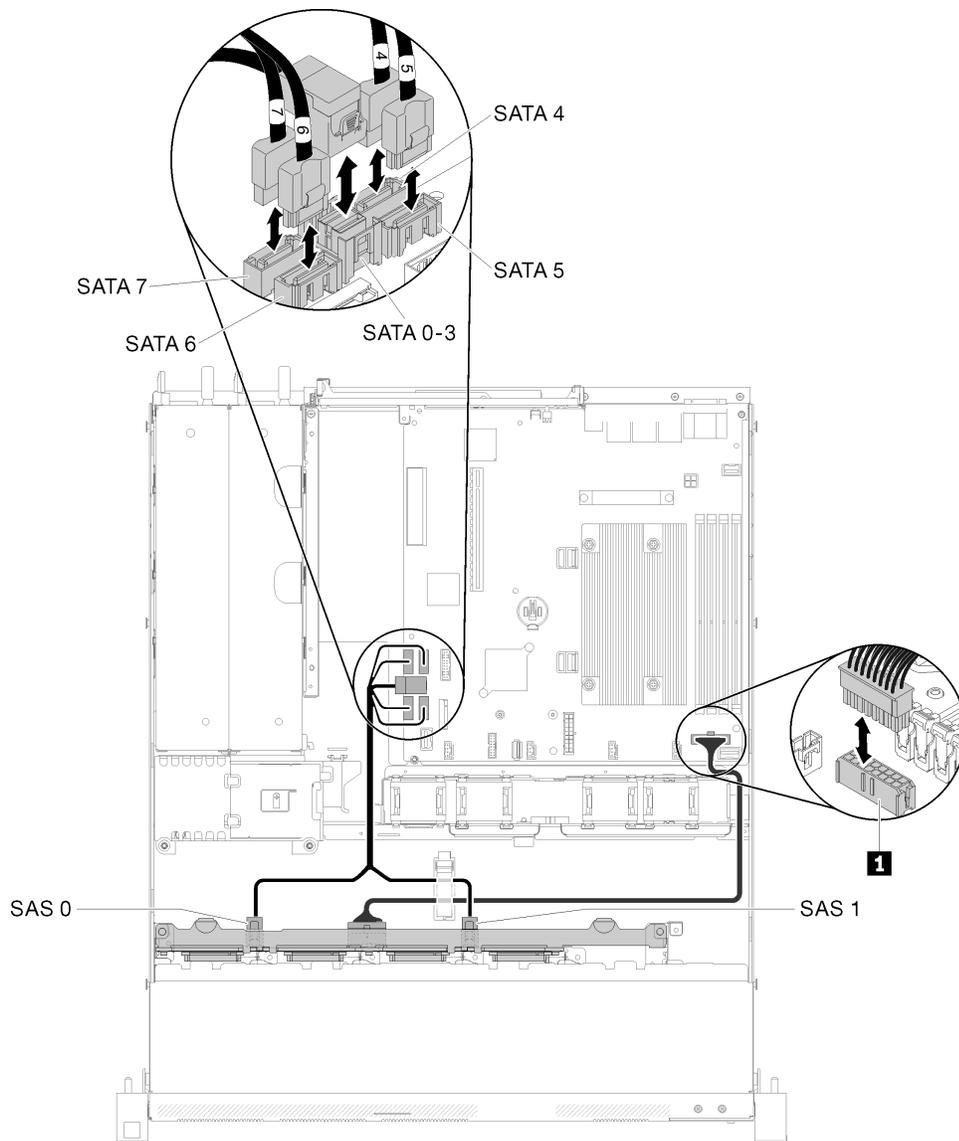
Figure 34. Eight 2.5-inch hot-swap drive model with software RAID
