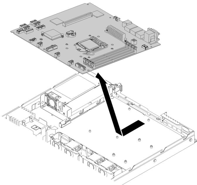
Figure 122. System board removal
