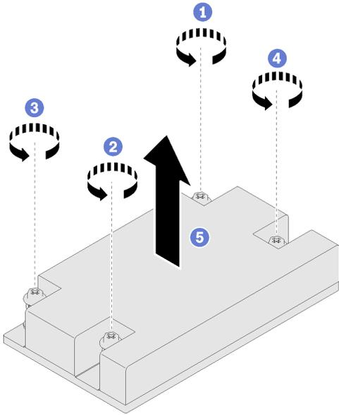
Figure 79. Heat sink removal
