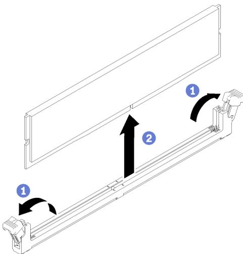
Figure 53. DIMM removal
