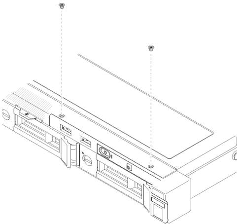
Figure 74. Front operator panel removal
