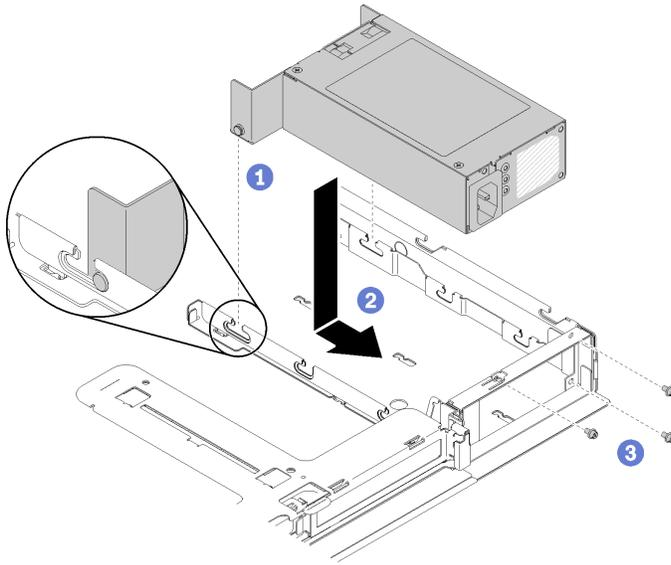
Figure 92. Power supply unit installation
