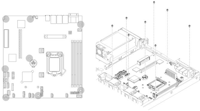
Figure 124. System-board screws location
