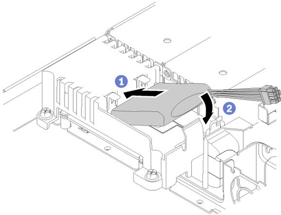
*Figure 66. Flash power module installation*
