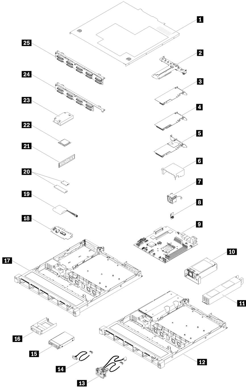
Figure 38. Server components - 2.5-inch drive model
