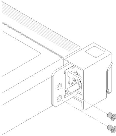
Figure 113. Rack latches installation
