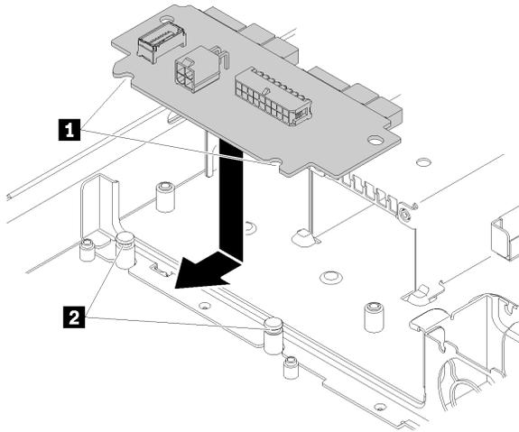
Figure 100. Power interface board installation
