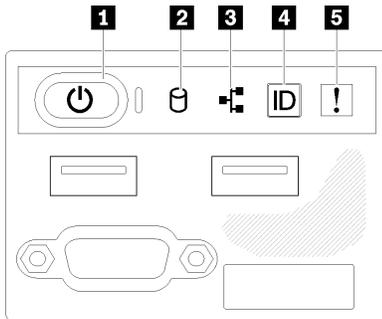
Figure 9. 2.5-inch drive chassis front I/O assembly
