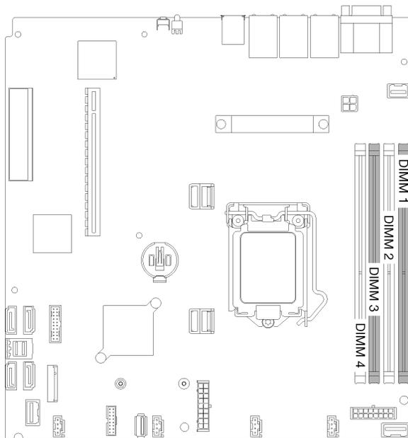
Figure 52. DIMM connectors
