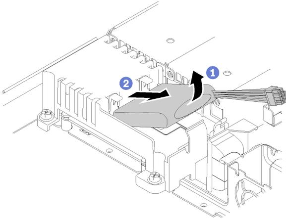
Figure 65. Flash power module removal
