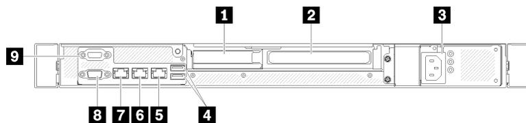
Figure 11. Rear view - Non-redundant power supply model
