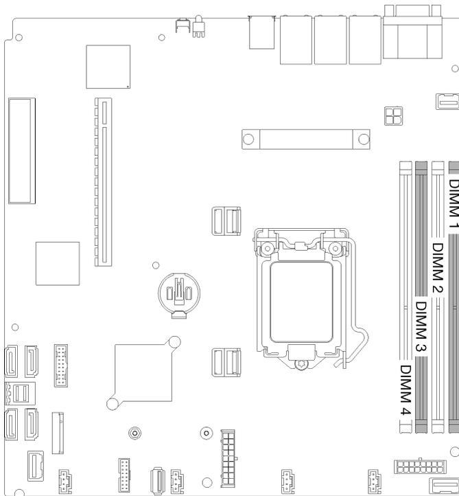
Figure 54. DIMM connectors
