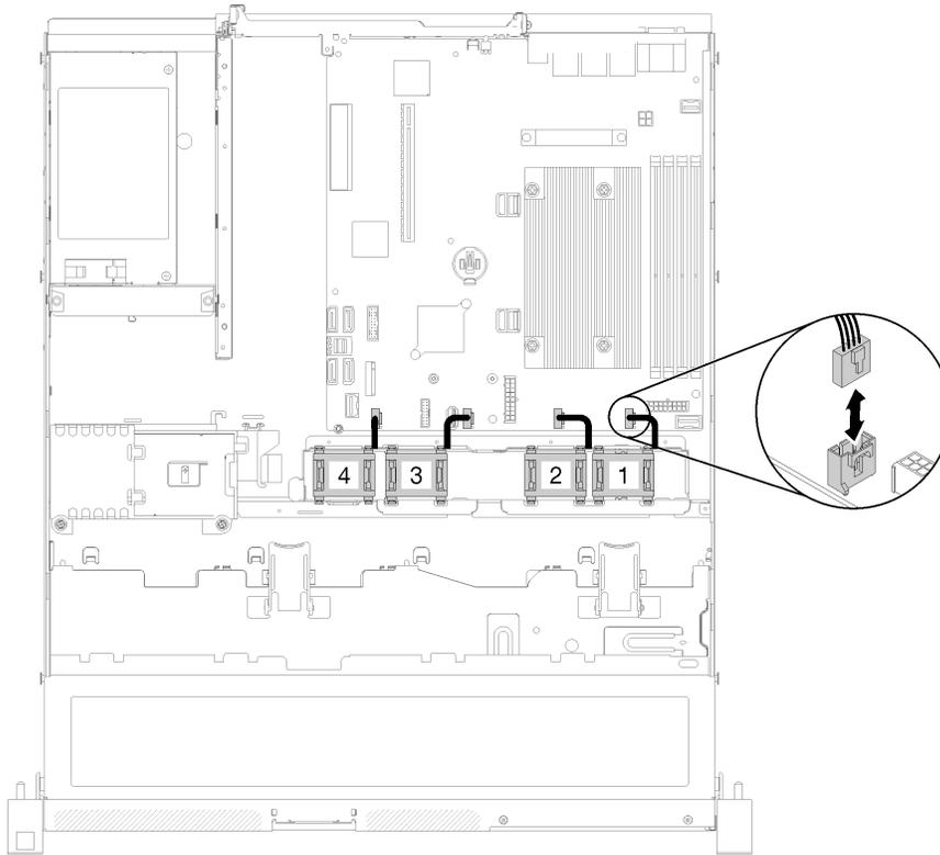
Figure 64. Fan power cable routing
