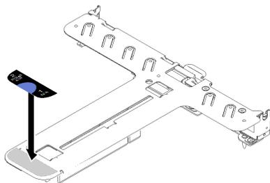
Figure 89. PCIe riser assembly installation
