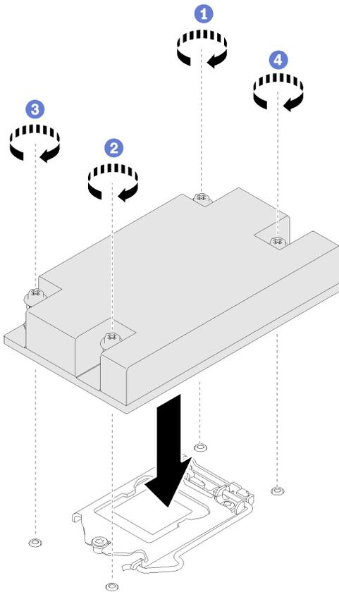
Figure 80. Heat sink installation
