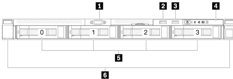
Figure 6. Four hot-swap drives model front view
