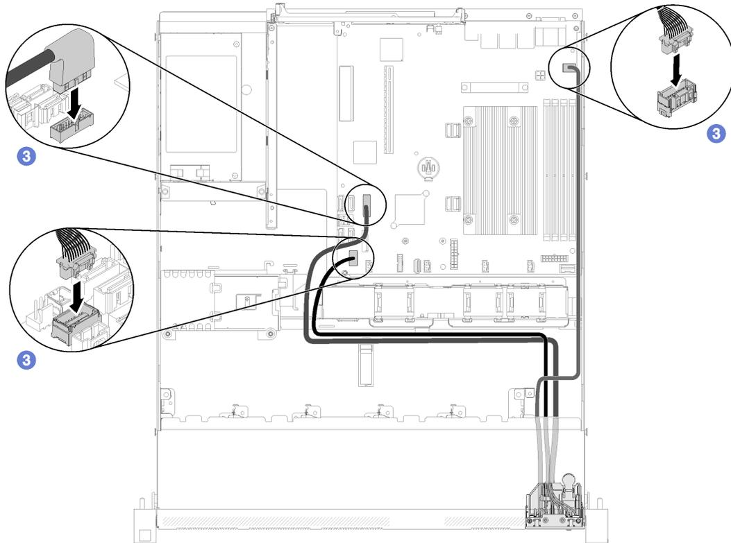
Figure 72. Front operator panel (2.5-inch HDD model) cable routing
