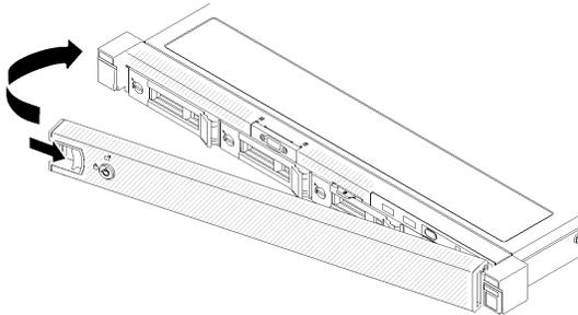
Figure 119. Security bezel installation
