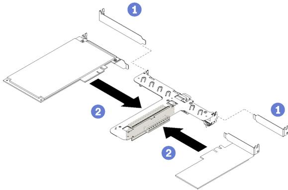
Figure 41. Adapter installation
