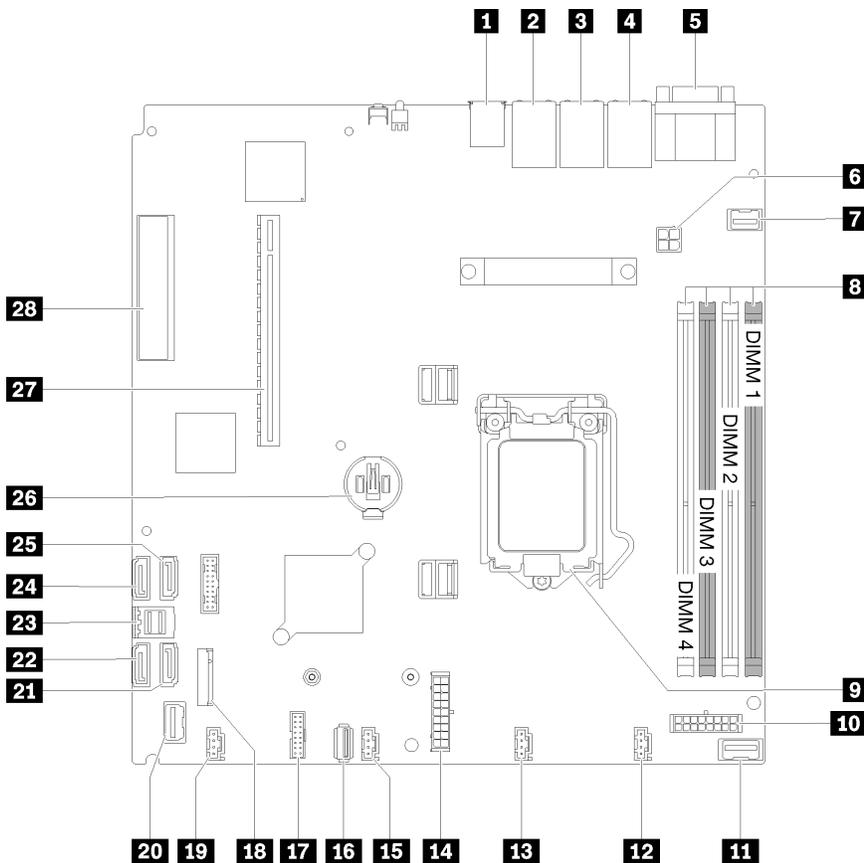
Figure 14. System-board connectors
