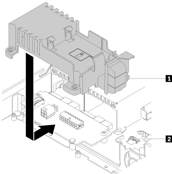
Figure 102. Power interface board cover installation
