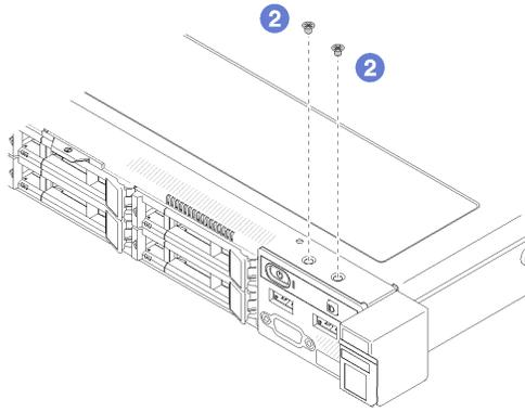
Figure 68. Screws removal
