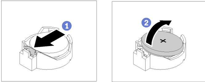
Figure 50. CMOS battery removal
