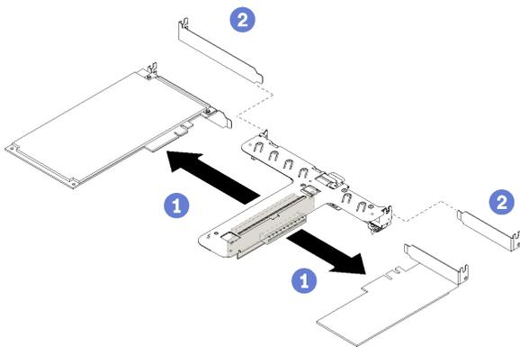
Figure 40. Adapter removal
