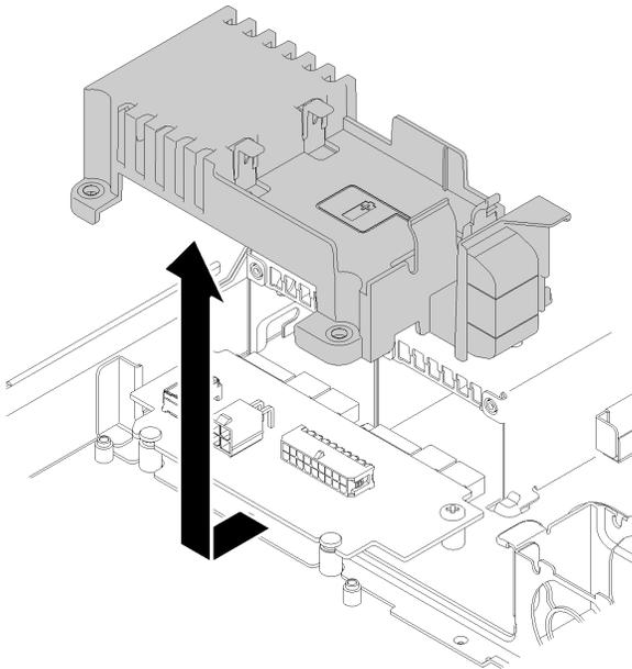
*Figure 97. Power interface board cover removal*
