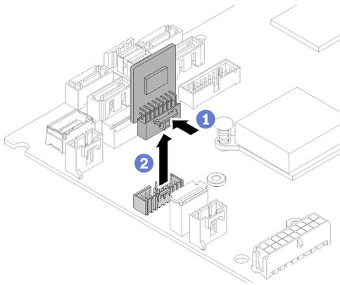
Figure 127. TPM card (for China only) removal
