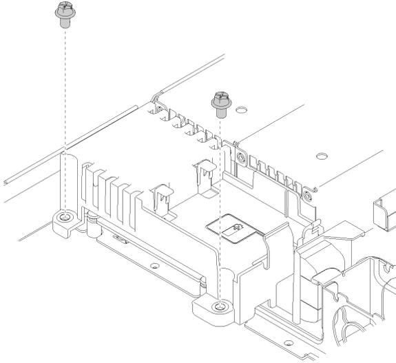
*Figure 96. Cover screw removal*
