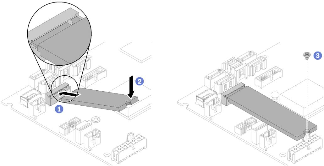
Figure 85. M.2 drive installation
