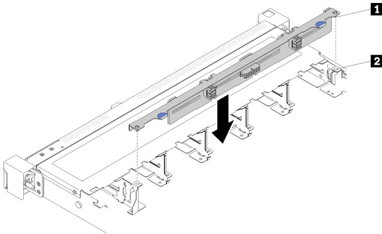
Figure 47. 3.5-inch hot-swap drive backplane installation
