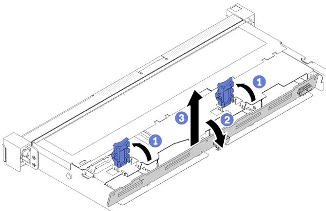
Figure 48. Backplate removal
