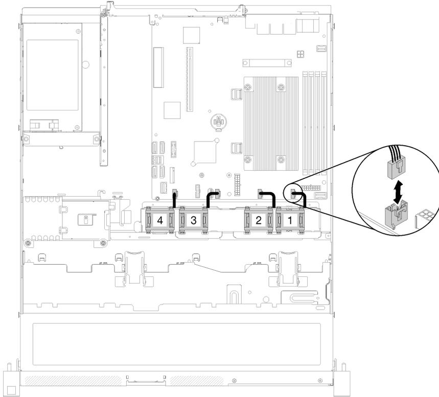
Figure 26. Fan cable routing
