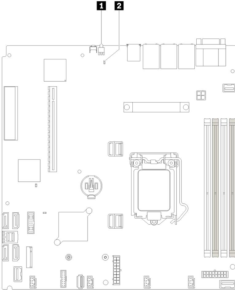
Figure 13. System-board LEDs
