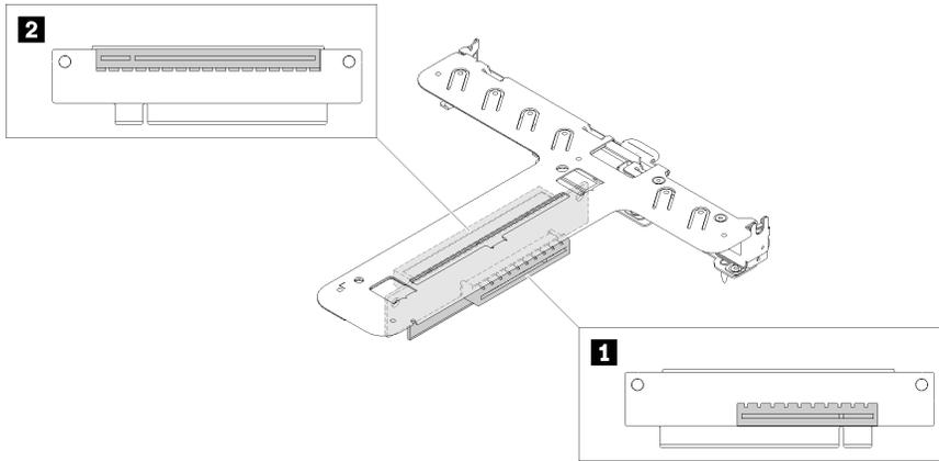
Figure 23. x8/x8 Butterfly riser assembly
