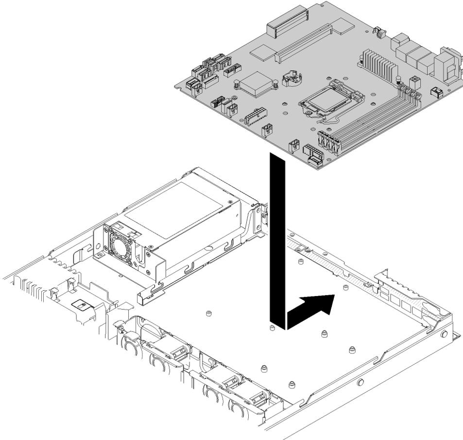
*Figure 123. System board installation*
