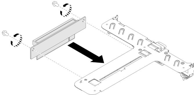
Figure 88. PCIe riser card installation
