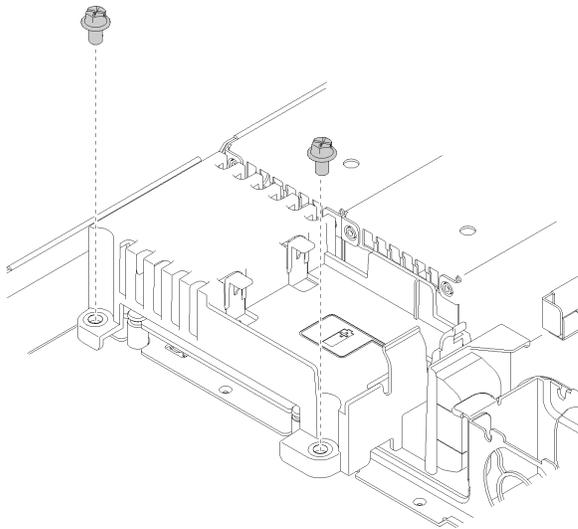
Figure 103. Cover screw installation
