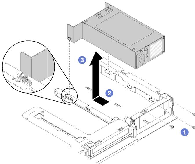
Figure 91. Power supply unit removal
