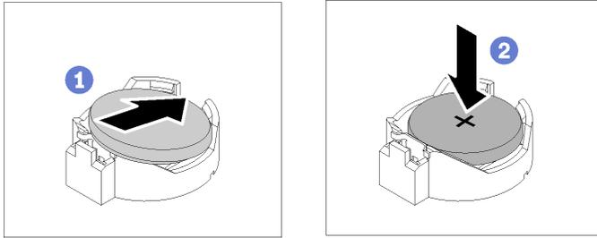
Figure 51. CMOS battery installation
