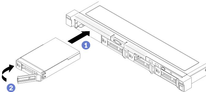
Figure 57. Simple-swap drive installation
