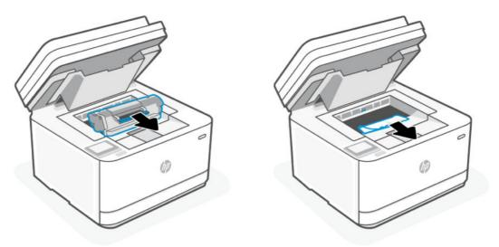
5. Reinstall the toner cartridge, lock the lever, and then close the cartridge access door.
