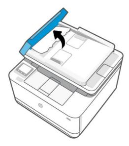
2. Remove any jammed paper. Use both hands to remove jammed paper to avoid tearing the paper.
