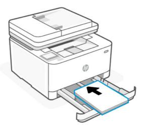
Make sure the stack of paper is aligned with the appropriate paper size lines in the tray. Also, make sure the stack of paper does not exceed the stack height marking in the tray.
