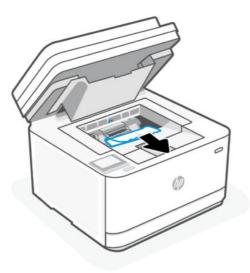
3. Release the lever and pull out the jammed paper.
