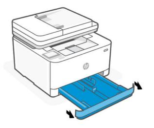
2. If you are loading Legal or longer paper, press the button near the front right of the tray to extend the input tray.
