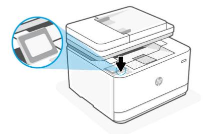
**NOTE:** Press down the control panel to return it to its original position.
