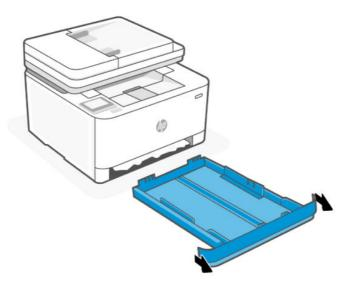
2. Check the input tray area underneath the printer. Remove the jammed paper.
