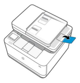
2. Slide the paper-width guides to the edges of the document feeder.
