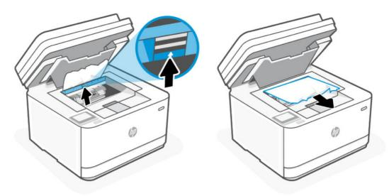
4. Remove the toner cartridge and pull out any jammed paper.
