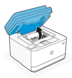
2. Before removing the cartridge, remove any jammed paper in the output tray area. If you can see the jammed paper, carefully grasp the jammed paper, and slowly pull it out of the output tray area.
