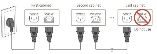
Transfer power by daisy chain with extension power cable.
