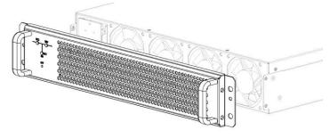
3. First Installation: Install the sponge board, sheet metal, washers and nuts. Maintenance: Replace a new sponge board to front cover. Recommendation Tool: Open jaw spanner 6mm
