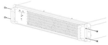
2. Remove the front cover from power module.
