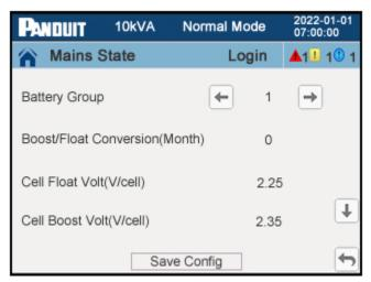
Figure 50: Battery Setting Page 1 (3-Phase UPS)
