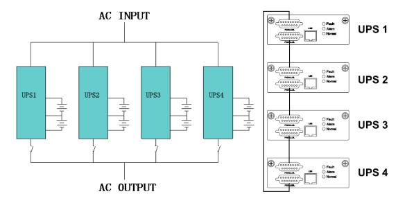
Figure 2: Parallel System Power/Control Connections
