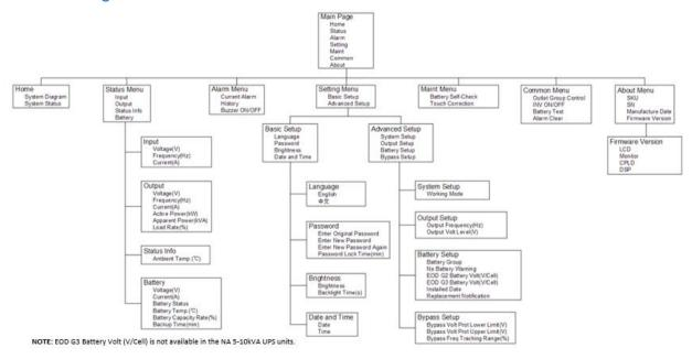
Figure 18: 5-10kVA Single-phase UPS Menu Structure
