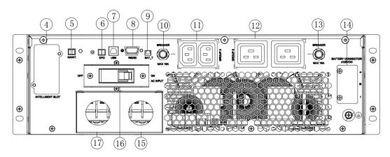
Figure 8: European 6-10kVA Rear View (U06N12V / U06S12V)
