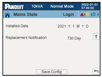
Figure 53: Battery Setting Page 2 (EU Single-Phase UPS)
