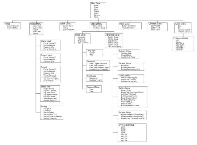
Figure 19: 10 – 20kVA 3-Phase UPS Menu Structure
