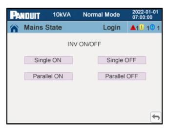
Figure 65: Inverter ON/OFF Page (3-Phase UPS)
