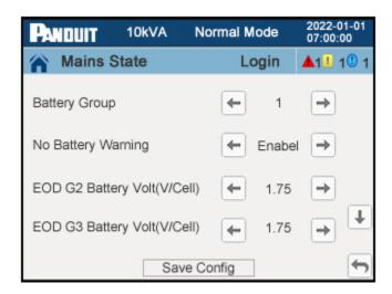
Figure 52: Battery Setting Page 1 (EU Single-Phase UPS)
