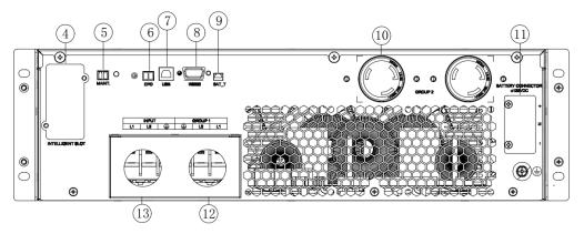
Figure 6: North American 5kVA Rear View (U05x11V)
