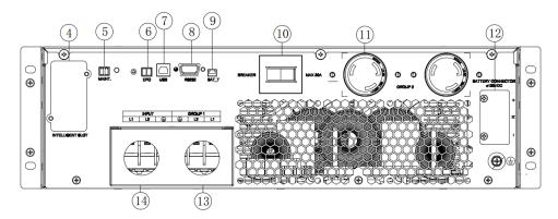
Figure 7: North American 6-10kVA Rear View (U06N11V / U06S11V)
