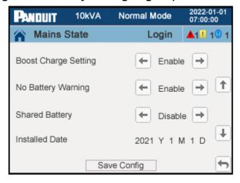
Figure 51: Battery Setting Page 2 (3-Phase UPS)
