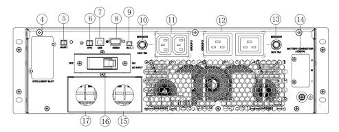
Figure 10: European 10kVA Rear View (U10N12V / U10S12V)
