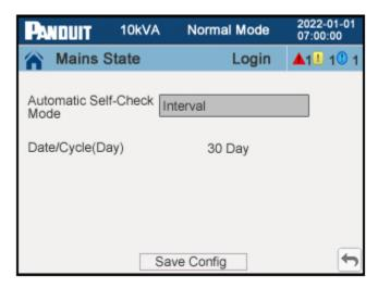
Figure 62: Auto Self-Check Interval Setting Page
