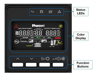
Figure 17: Front Panel Display (FPD)
