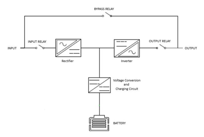
Figure 1: High-level Double Conversion UPS Block Diagram
