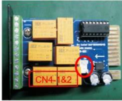
Figure 16: Relay Card Front and Top View (showing connection points)
