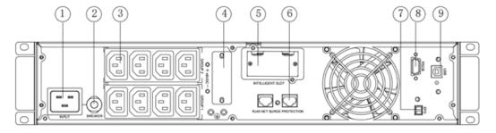
Figure 8: 2kVA EU Rear Panel View
