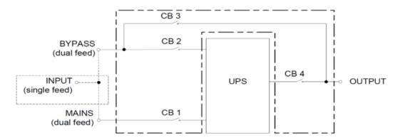
Figure 13: High-level Maintenance Bypass Switch Block Diagram
