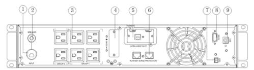
Figure 4: 1kVA NA Rear Panel View
