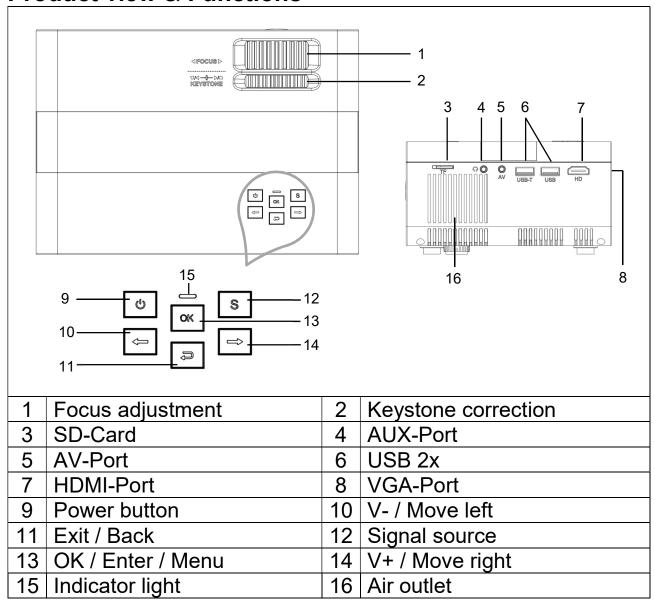
Power button: Press this button to shut on or off the device.
