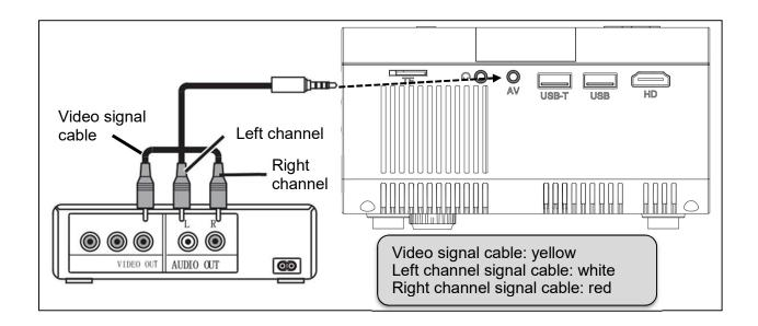
**Audio output:** Audio signal from the output port of the device, if you want to high powerplay music input end connected to external power amplifier.
