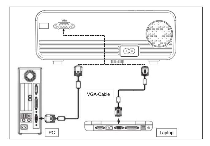
**NOTE:** The device and connection of laptop may not be able to display images at the same time, if that happens, set the computer display attributes, select for CRT output mode.
