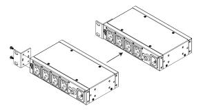
3. Align the unit and the rack mount ear to the rack and stabilize the unit using rack screws. Let the buttons stabilize in the button holes and the mounting is complete.
