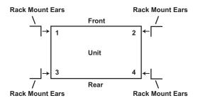
2. Align and stabilize the rack mount ear using M3 Phillips hex screws.
