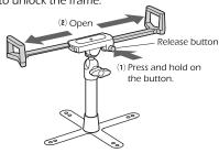
2. Install the tablet PC on the frame.
