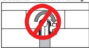
DO NOT attempt to adjust, tilt, or rotate any ball socket joints while it is fully tightened. Any such action will result in possible damage and loss of integrity of product functioning at full capacity. Manufacturer will not be responsible for any such actions by any person.
