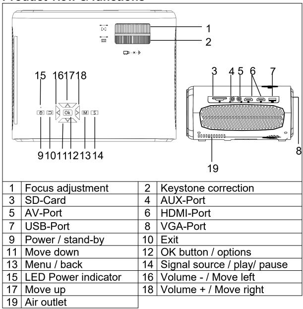
**Power button:** Press this button to power on the device. To set the projector in stand-by, press twice.
