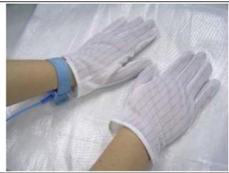
Hold LCD by the side carefully and DON'T touch or press panel directly.
