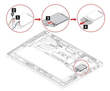
**Note:** During installation, ensure that you connect the cables with different colors to the corresponding connectors on the card according to the illustrations above: the orange cable to the connector labeled ORANGE, the blue cable to the connector labeled BLUE, the white and grey cable to the connector labeled WHITE GREY, and the black and grey cable to the connector labeled BLACK GREY.
