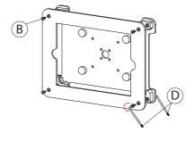
1B.While holding the back security star key (D) tight in place Turn the front security star key (D) counter clock-wise until all 4 Screws(B) are unscrewed.
