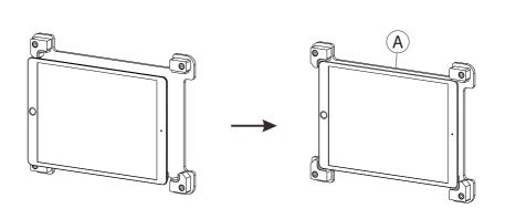
2A. Using one of the compatible listed tablets, insert into the foam adapters for a secure and tight fit. Insert tablet in back part of enclosure (A) as shown. Watch out orientation of tablet.
