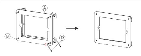
3A. Take the detached enclosure top (A), align the corner holes with the bottom portion. Then use the provided security star key (D), turn in clock-wise the star screws until securely tightened while holding the security star key (D) on the other side with your other hand. Screw in until securely tightened.
