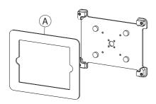
1C. Separate front part of enclosure (A) as shown.
