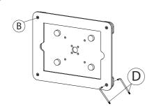
1A. Align the security star keys x2 (D) and insert it one in the front screw (B) and one in the Back screw (C) as shown.
