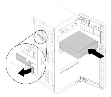
Figure 122. Installing a tape drive
