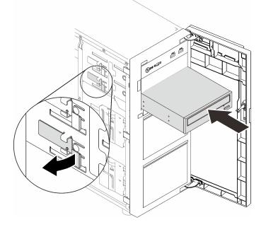
Figure 89. Installing an optical drive
