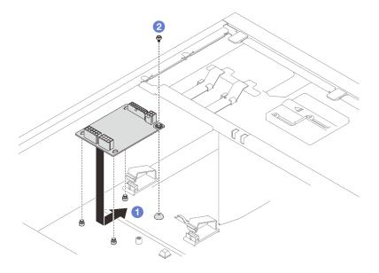
Figure 93. Installing the power distribution board of the fixed power supply
