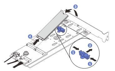
Figure 75. Removing an M.2 drive
