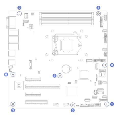
Figure 120. Tightening the screws to secure the system board
