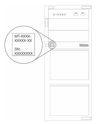
Figure 4. Location of the machine type, model, and serial number
