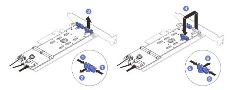
Figure 76. Adjusting the M.2 retainer
