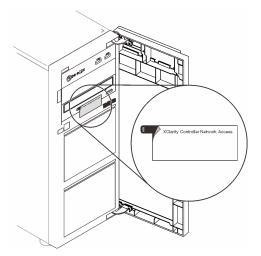
Figure 2. Location of the XClarity Controller network access label
