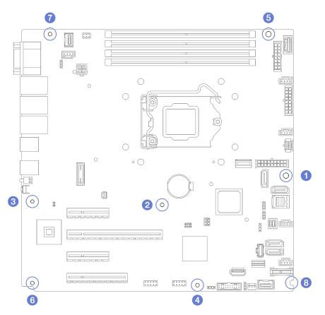
Figure 118. Removing the screws that secure the system board
