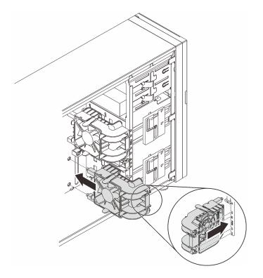
Figure 54. Installing the front system fan
