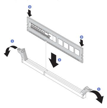
Figure 85. Installing a memory module
