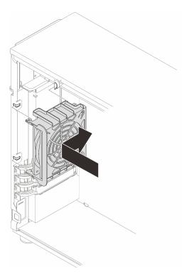
Figure 56. Positioning the rear system fan into the chassis
