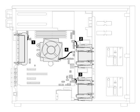
Figure 22. Fan power cable routing
