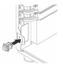
Figure 67. Installing the intrusion switch
