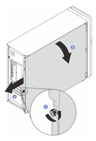
Figure 115. Removing the server cover
