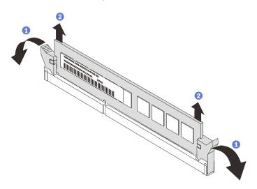
Figure 81. Removing a memory module
