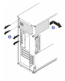
Figure 98. Removing a fixed power supply
