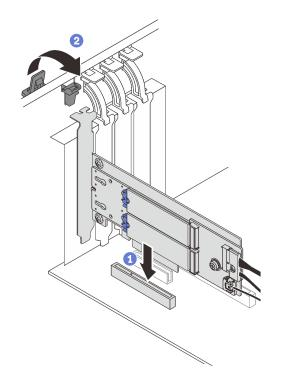
Figure 74. Installing the PCIe adapter into the chassis
