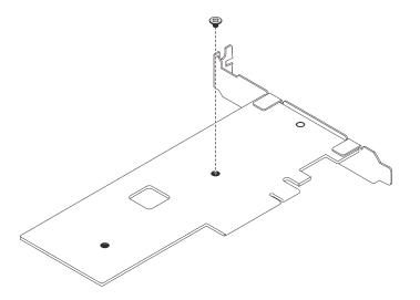
Figure 71. Removing the screw on the back of the PCIe adapter
