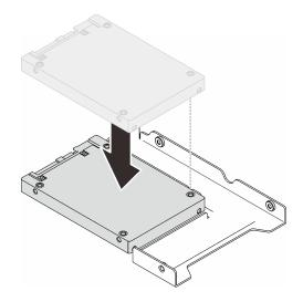
Figure 50. Positioning the 2.5-inch drive into the drive adapter
