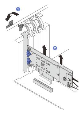
Figure 68. Removing the PCIe adapter that secures the M.2 boot adapter
