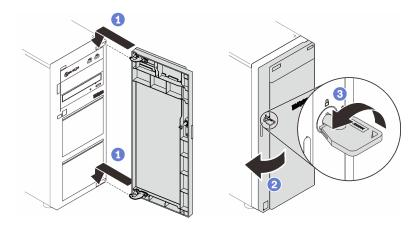
Figure 61. Installing the front door
