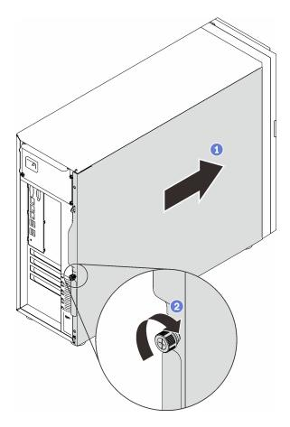
Figure 117. Securing the server cover to the chassis
