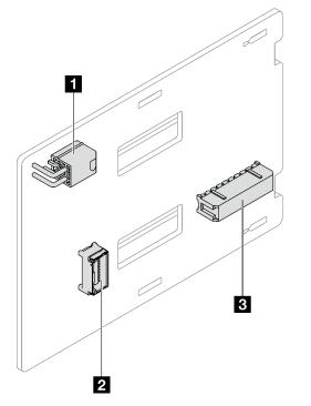
Figure 15. Power distribution board for hot-swap power supplies
