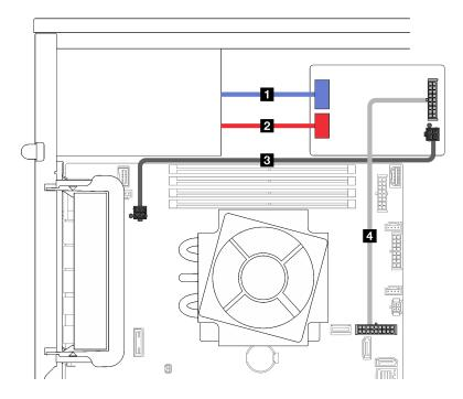
Figure 29. Cable routing for the fixed power supply
