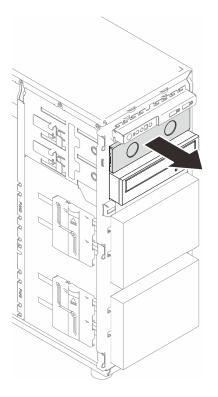
Figure 88. Removing the EMI shield from the optical drive bay
