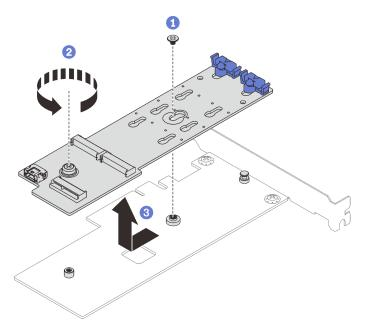
Figure 70. Removing the M.2 boot adapter
