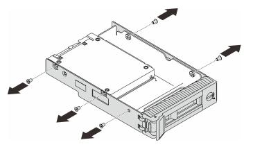
Step 4. Remove the two screws that secure the 2.5-inch drive; then, lift the drive to remove it from the drive adapter.
