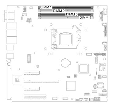
Figure 83. Memory module slots on the system board
