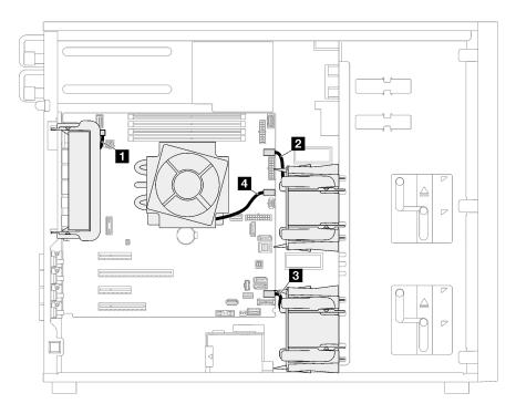
Figure 27. Fan power cable routing
