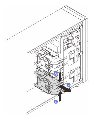
Figure 53. Removing the front system fan
