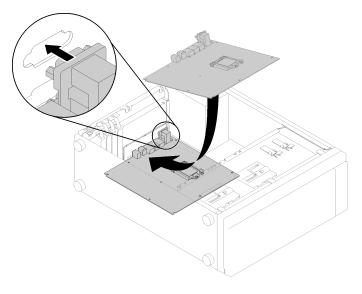
Figure 119. Installing the system board
