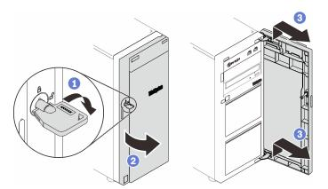
Figure 60. Removing the front door
