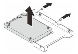
Figure 49. Removing the 2.5-inch drive from the drive adapter
