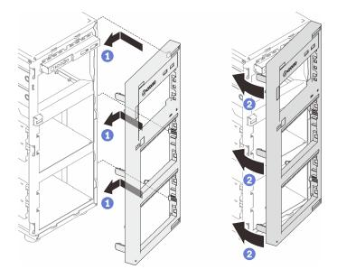
Figure 59. Installing the front bezel
