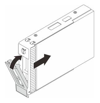
Figure 47. Installing the simple-swap drive
