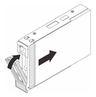
Figure 44. Installing the hot-swap drive
