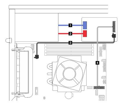
Figure 24. Cable routing for the fixed power supply
