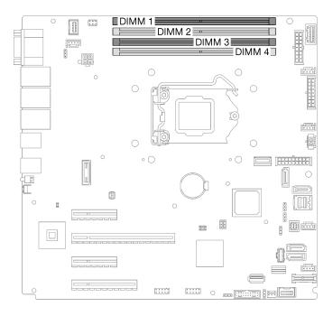
Figure 82. Memory module slots on the system board
