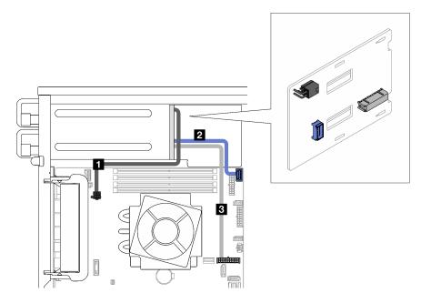
Figure 25. Cable routing for the redundant power supplies
