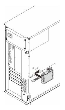
Figure 114. Installing the RAID flash power module and bracket assembly onto the chassis
