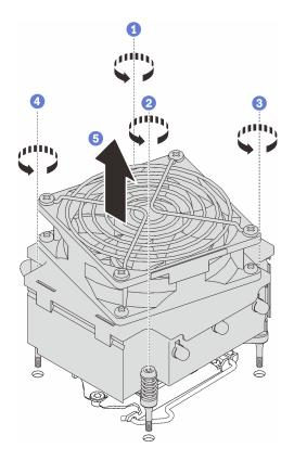
Figure 64. Removing the heat sink and fan module
