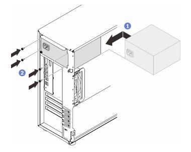
Figure 101. Installing a fixed power supply
