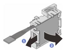
Figure 112. Removing the RAID flash power module from the bracket
