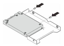
Figure 51. Installing the screws to secure the drive to the drive adapter
