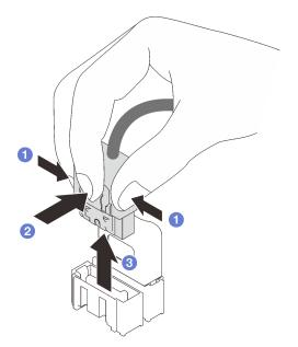
Step 3. Remove the drive cage from the chassis (see "Remove the 3.5-inch/2.5-inch drive cage" on page 88).
