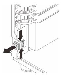
Figure 66. Removing the intrusion switch
