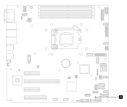
Figure 12. System-board LED
