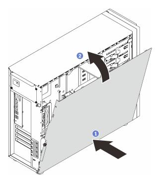
Figure 116. Positioning the server cover onto the chassis
