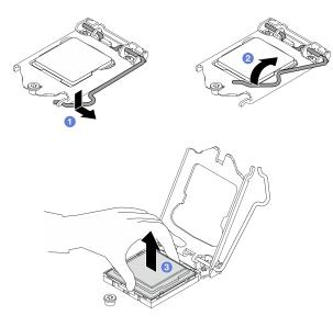
Figure 107. Opening the processor retainer
