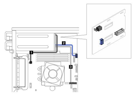
Figure 30. Cable routing for the redundant power supplies
