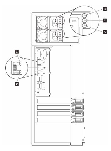
Figure 10. Rear view LEDs of the server
