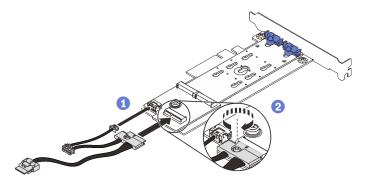
Figure 73. Installing the M.2 power and signal cables
