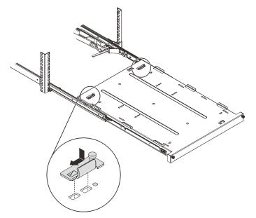
Step 4. Install the four rubber safety pads as illustrated.
