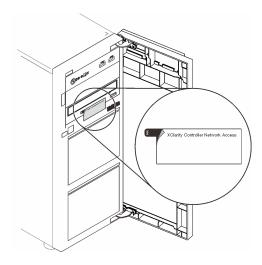
Figure 5. Location of XClarity Controller network access label
