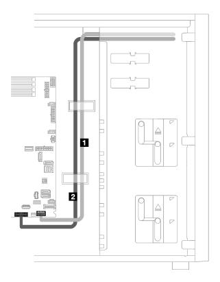
Figure 23. Cable routing for the front panel
