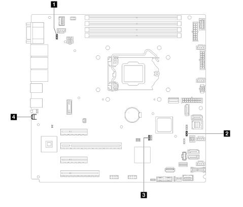
Figure 13. System-board jumpers and buttons
