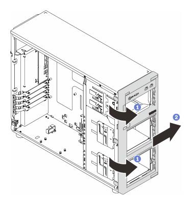
Figure 58. Removing the front bezel
