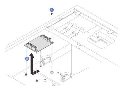
Figure 92. Removing the power distribution board of the fixed power supply
