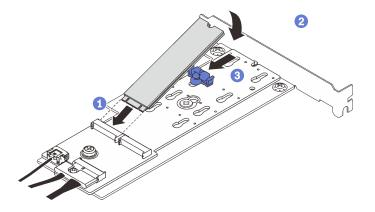
Figure 78. Installing an M.2 drive
