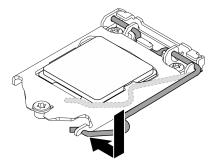
Figure 110. Closing the processor retainer
