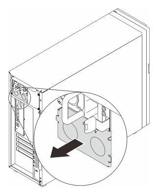
Figure 105. Removing a hot-swap power supply filler
