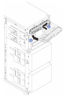
Figure 63. Installing the front panel board assembly
