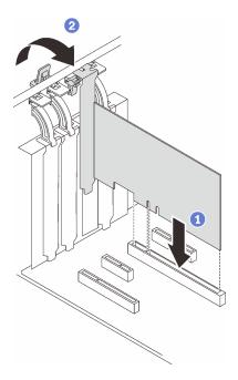
Figure 91. Installing a PCIe adapter
