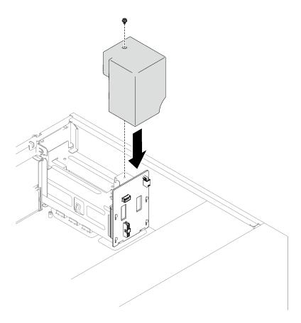
Figure 96. Installing the power distribution board cover
