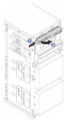
Figure 62. Removing the front panel board assembly
