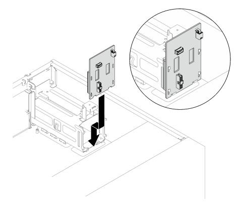
Figure 95. Installing the power distribution board of the hot-swap power supply
