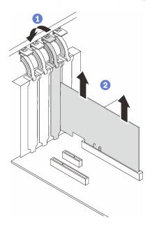
Figure 90. Removing a PCIe adapter
