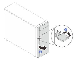
Step 2. Lift the front door to detach the hinge, and remove it from the server.
