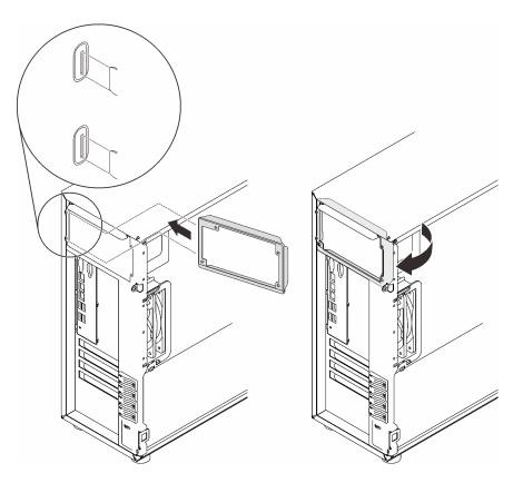
Figure 100. Installing a fixed power supply bracket
