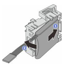
Figure 113. Installing the RAID flash power module into the bracket
