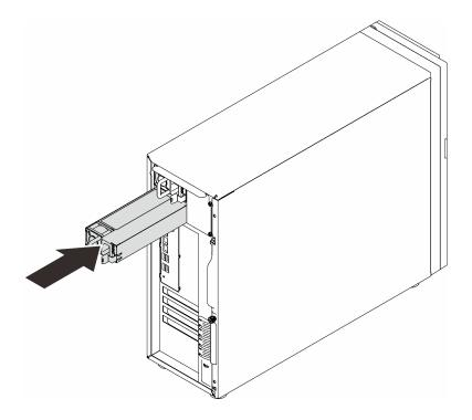
Figure 106. Installing a hot-swap power supply
