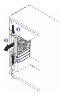
Figure 55. Removing the rear system fan
