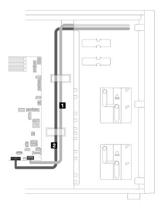
Figure 28. Cable routing for the front panel
