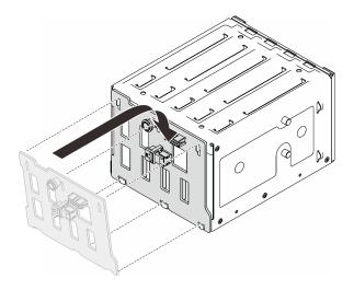
Figure 36. Installing the hot-swap drive backplane
