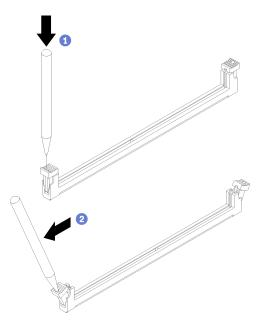
Figure 84. Opening retaining clips
