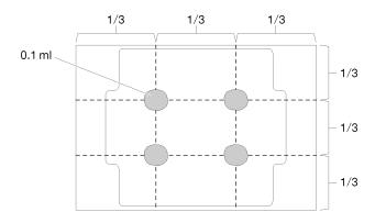
Figure 108. Proper shape of the thermal grease
