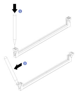
Figure 80. Opening retaining clips
