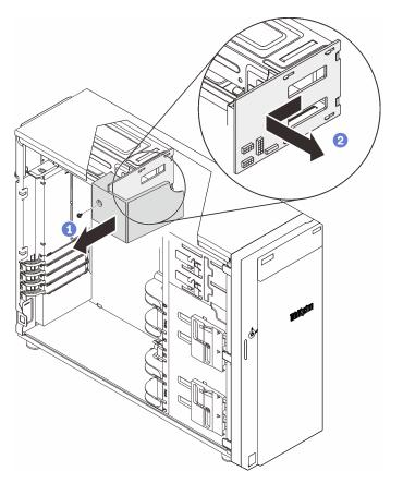
Figure 94. Removing the power distribution board of the hot-swap power supply
