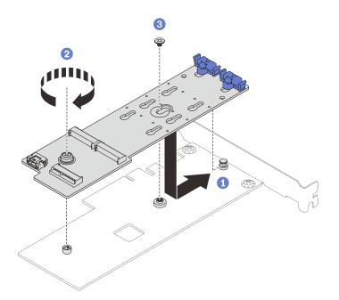
Figure 72. Securing the M.2 boot adapter to the PCIe adapter
