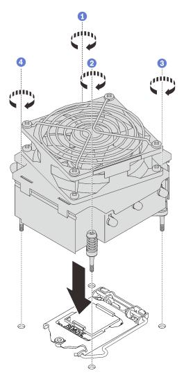
Figure 65. Installing the heat sink and the fan module
