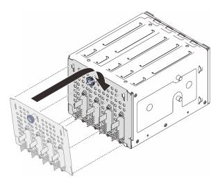
Figure 39. Installing the simple-swap drive backplate
