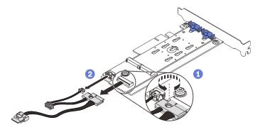
Figure 69. Disconnecting the power and signal cables
