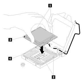
Figure 109. Installing the processor
