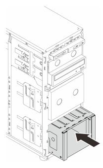
Figure 33. Installing the drive cage
