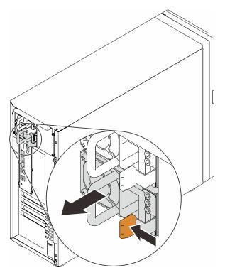
Figure 103. Removing a hot-swap power supply
