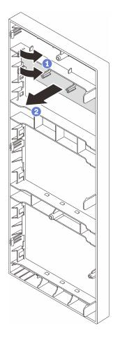
Figure 87. Removing the plastic bay filler from the optical drive bay
