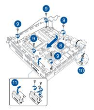
11. Replace the configurable port and secure it to the Mini PC using the three (3) screws removed previously.
