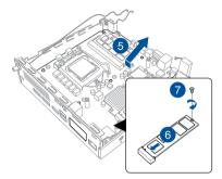
8. After installing the M.2 SSD, flip the motherboard over again and replace the motherboard into the chassis.
