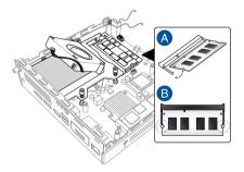
6. Flip the fan over towards the front of the chassis so that the fan rests over the installed memory modules, then secure it with the three (3) screws previously removed.
