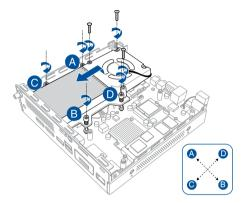
6. Reconnect the CPU fan cable (A) and WiFi antenna cables (B).
