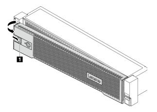
Figure 284. Security bezel removal
