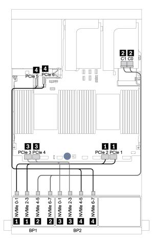
Figure 55. Cable routing for 16 x 2.5-inch NVMe configuration with one retimer card
