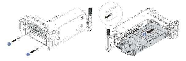
Figure 274. 7mm drive cage removal
