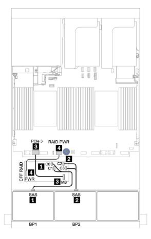
Figure 40. Cable routing for 16 x 2.5-inch SAS/SATA configuration with one CFF 16i RAID/HBA adapter
