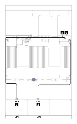
Figure 39. Cable routing for the 16 x 2.5-inch SAS/SATA configuration with two 8i RAID/HBA adapters or one 16i/32i RAID/HBA adapter
