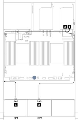
Figure 94. Cable routing for the 8 x 2.5-inch SAS/SATA + 8 x 2.5-inch Anybay configuration with one 8i/16i RAID/HBA adapter and one Trimode 8i RAID adapter
