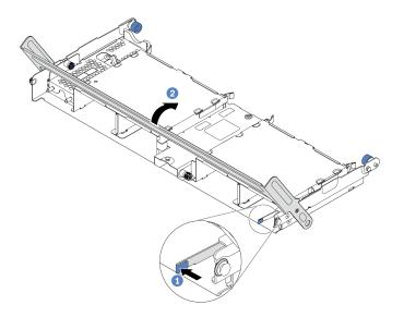
Figure 200. Closing the drive cage handle
