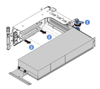
Figure 165. Removing the GPU adapter
