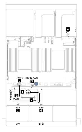
Figure 95. Cable routing for the 8 x 2.5-inch SAS/SATA + 8 x 2.5-inch Anybay configuration with one CFF 16i RAID/HBA adapter and one Trimode 8i RAID adapter
