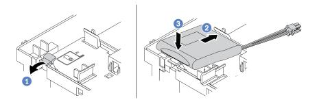
Figure 247. Super capacitor installation on the air baffle
