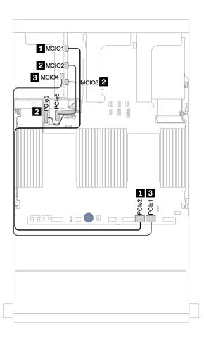
Figure 22. Cable routing for x16/x16 PCIe riser card 3 (configuration with 32 NVMe drives)
