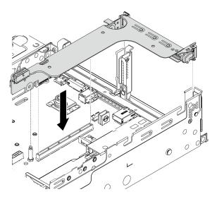
Figure 299. Installing the riser assembly
