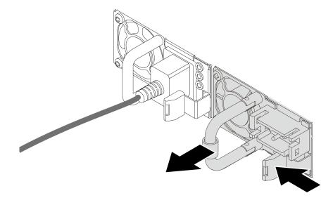
Figure 217. Hot-swap power supply removal
