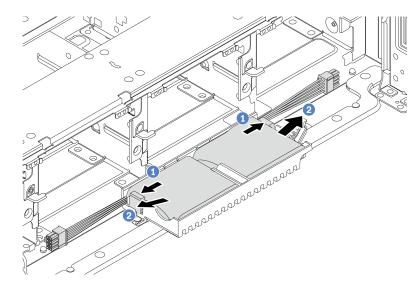
Figure 242. Super capacitor module removal
