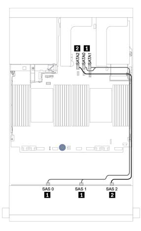
Figure 131. Cable routing for the 12 x 3.5-inch SAS/SATA configuration with onboard connectors
