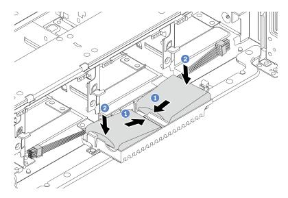
Figure 245. Super capacitor module installation
