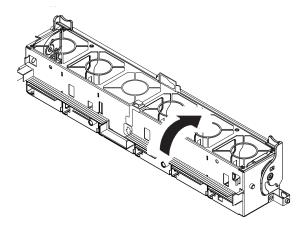
Step 3. Install the intrusion switch onto the fan cage.
