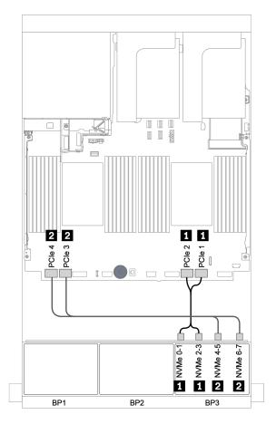
Figure 108. NVMe cable routing
