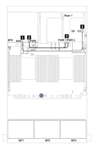
Figure 112. Cable routing for the rear 4 x 2.5-inch SAS/SATA backplane
