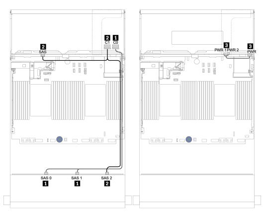
Figure 126. Cable routing for the 12 x 3.5-inch SAS/SATA configuration with a 4 x 3.5-inch SAS/SATA rear backplane
