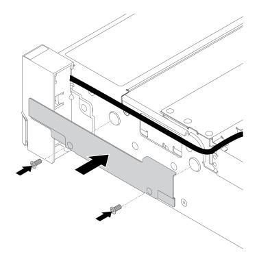
Figure 236. Cable retainer installation
