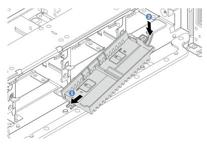
Figure 244. Super capacitor holder installation
