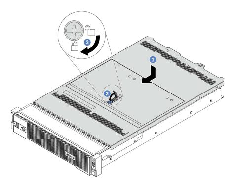
Figure 303. Top cover installation
