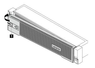
Figure 286. Security bezel installation
