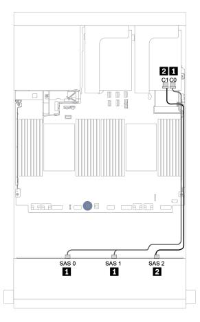
Figure 121. Cable routing for the 12 x 3.5-inch SAS/SATA configuration with one 16i RAID/HBA adapter
