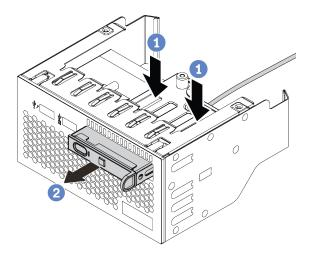
Figure 159. LCD diagnostic panel removal
