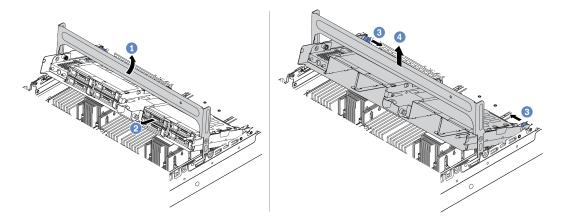
Figure 199. Removing the middle drive cage and drives
