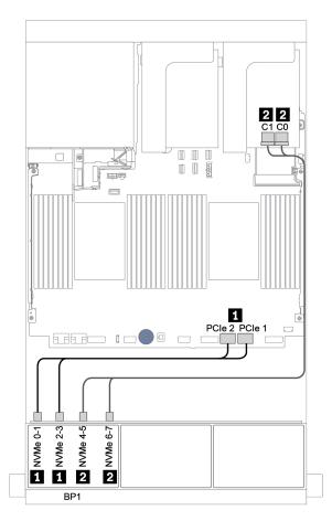
Figure 54. Cable routing for the 8 x 2.5-inch NVMe configuration with one retimer card
