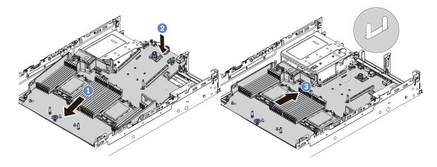
Figure 289. System board installation
