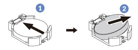
Figure 154. CMOS battery removal
