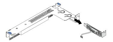
Figure 295. Removing the riser bracket
