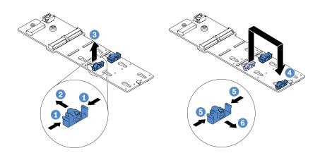
Figure 192. M.2 retainer adjustment
