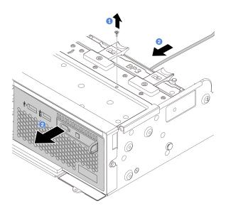
Figure 158. Front I/O assembly removal
