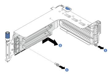
Figure 212. Riser card removal
