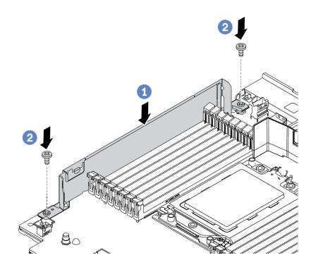
Figure 153. Cable wall brackets installation
