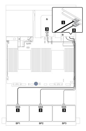
Figure 41. Cable routing for the 24 x 2.5-inch SAS/SATA configuration with three 8i RAID/HBA adapters
