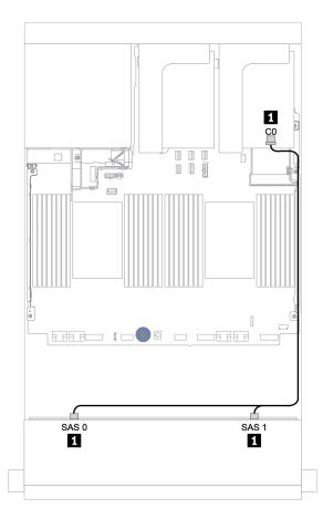
Figure 119. Cable routing for the 8 x 3.5-inch SAS/SATA configuration with one 8i RAID/HBA adapter
