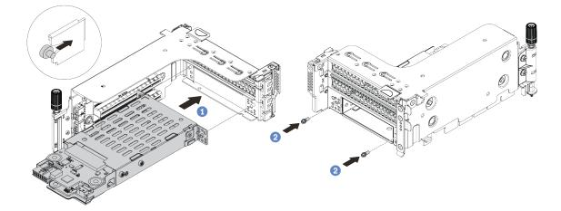
Figure 281. 7mm drive cage installation
