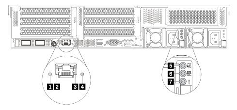
Figure 10. Rear view LEDs of the server
