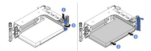
Figure 211. PCIe adapter removal
