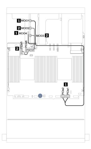
Figure 21. Cable routing for x16/x16 PCIe riser card 3
