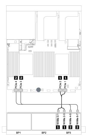
Figure 105. NVMe cable routing (two processors)
