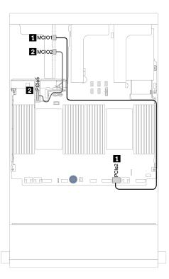
Figure 19. Cable routing for x8/x8 PCIe riser card 3
