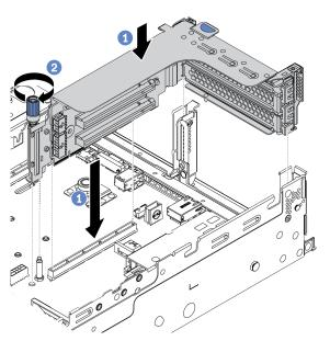
Figure 215. Riser assembly installation
