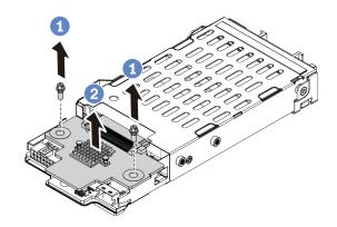
Figure 276. 7mm drive backplane removal (top)
