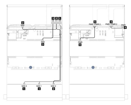
Figure 133. Cable routing for the 12 x 3.5-inch SAS/SATA + 4 x 3.5-inch SAS/SATA + 4 x 3.5-inch SAS/SATA configuration with one 32i RAID/HBA adapter
