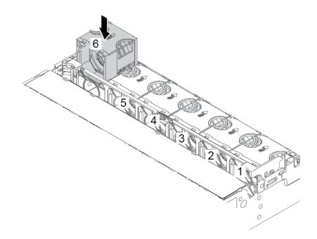
Figure 291. System fan installation
