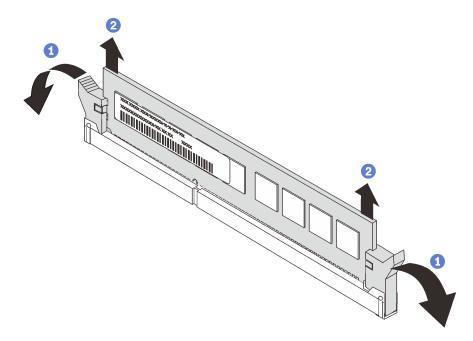
Figure 196. Memory module removal
