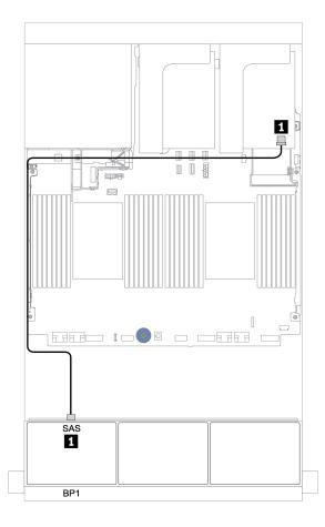
Figure 36. Cable routing for the 8 x 2.5-inch SAS/SATA configuration with one 8i/16i RAID/HBA adapter
