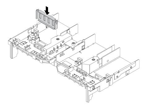
Figure 169. Installing the GPU air baffle filler
