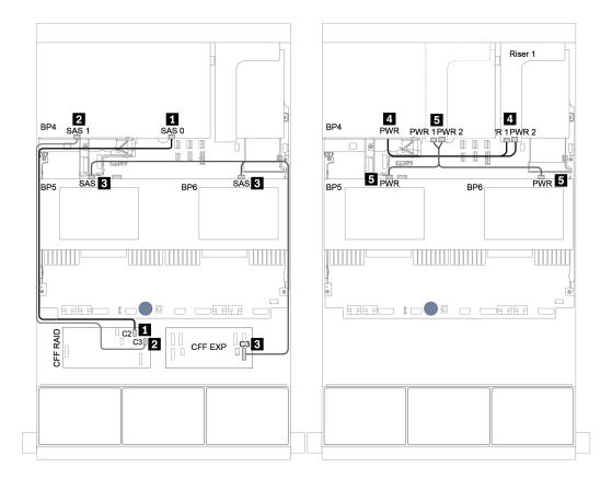
Figure 52. Cable routing for middle 4 x 2.5 SAS/SATA backplanes and rear 8 x 2.5 SAS/SATA backplane
