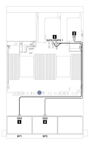
Figure 93. Cable routing for the 8 x 2.5-inch SAS/SATA + 8 x 2.5-inch Anybay configuration with one Trimode 8i RAID adapter
