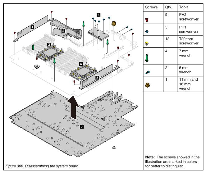
Step 1. Remove the system board from the server (see "Remove the system board" on page 354).
