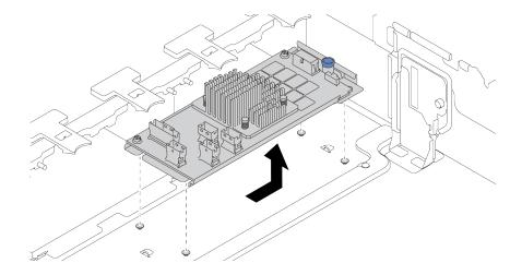
Figure 183. Internal CFF adapter removal
