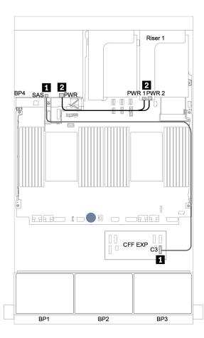
Figure 50. Cable routing for the 4 x 2.5-inch SAS/SATA rear backplane
