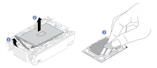
Figure 223. Separating a processor from the heat sink and carrier
