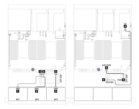
Figure 46. Cable routing for the 24 x 2.5-inch SAS/SATA configuration with one CFF expander and one 8i RAID/HBA adapter
