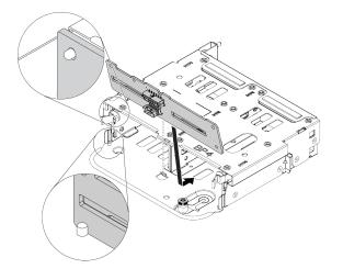
Figure 261. Installing the 4 x 2.5-inch rear drive backplane
