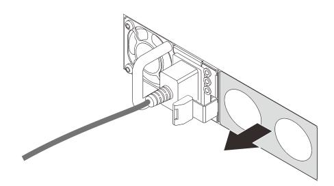
Figure 219. Hot-swap power supply filler removal
