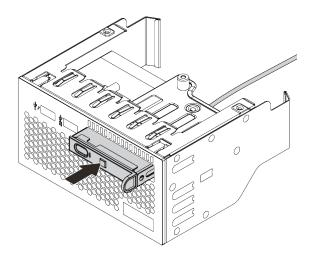
Figure 161. LCD diagnostics panel installation
