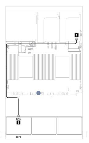
Figure 82. Cable routing for the 8 x 2.5-inch Anybay configuration with one Trimode 8i RAID adapter
