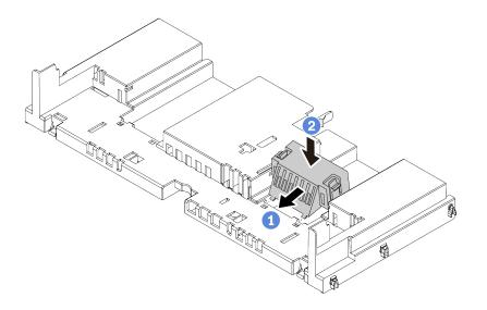
Figure 150. Air baffle filler removal
