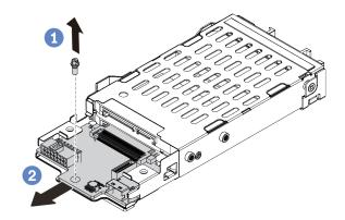
Figure 277. 7mm drive backplane removal (bottom)
