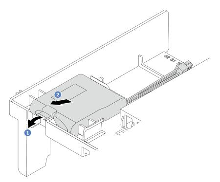
Figure 246. Super capacitor module removal
