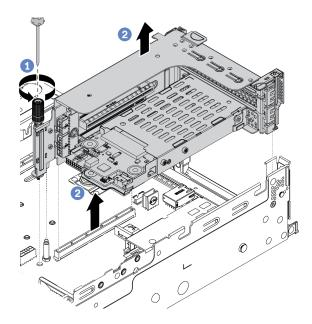
Figure 273. Riser assembly removal
