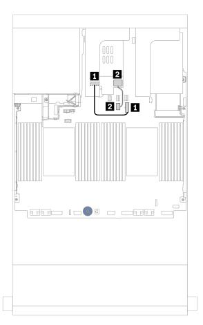
Figure 28. Cable routing for 7mm drives
