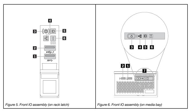
**Note:** The LCD diagnostic panel **1** on media bay provides an LCD display to quickly access system information such as active errors, system status, firmware information, network information, and health information. For details, see "LCD diagnostics panel" on page 29.
