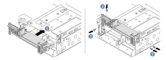
Figure 256. C1 rearwall bracket installation (right)
