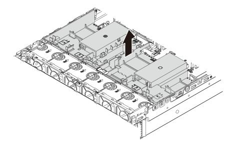
Figure 148. Air baffle removal
