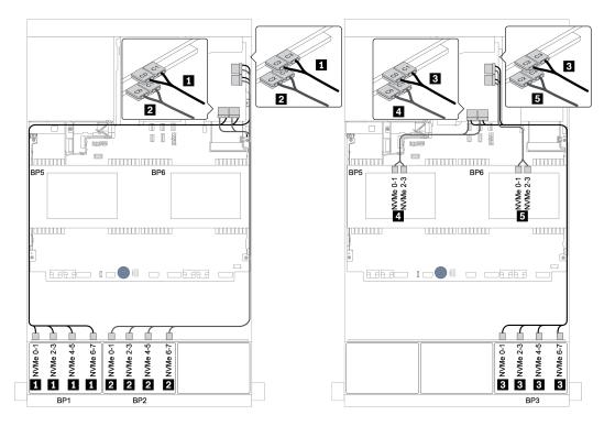
Figure 57. Cable routing for the 32 x 2.5-inch NVMe configuration with four switch cards
