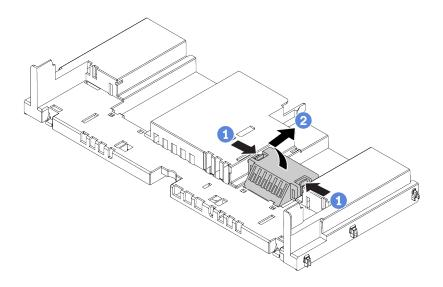
Figure 149. Air baffle filler removal
