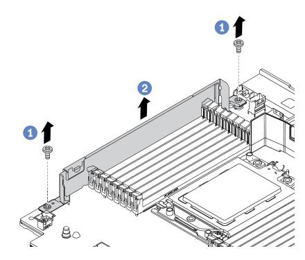
Figure 152. Cable wall brackets removal
