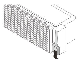
Figure 230. ID label plate removal
