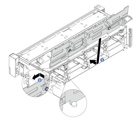
Figure 182. 3.5-inch drive backplane installation
