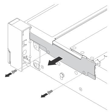
Figure 231. Cable retainer removal
