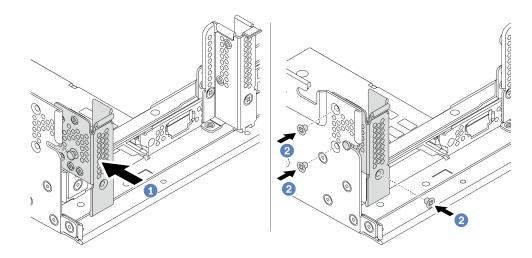
Figure 254. A1 rearwall bracket installation (left)
