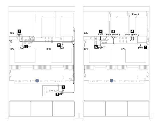
Figure 51. Cable routing for the 4 x 2.5-inch SAS/SATA middle backplanes and 4 x 2.5 SAS/SATA rear backplane
