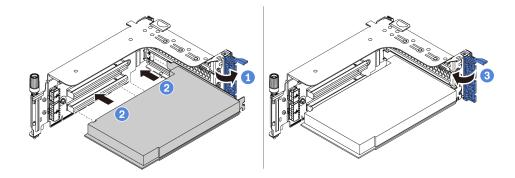
Figure 214. PCIe adapter installation
