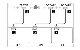
Figure 34. Power cable connections for 8 x 2.5-inch drive backplanes
