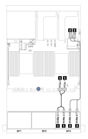
Figure 114. NVMe cable routing (one processor)
