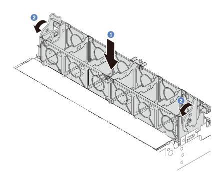
Figure 293. System fan cage installation
