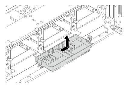
Figure 243. Super capacitor holder removal
