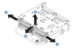
Figure 259. Removing the rear 4 x 2.5-inch drive backplane
