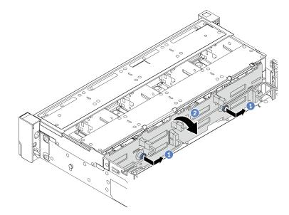
Figure 181. 3.5-inch drive backplane removal
