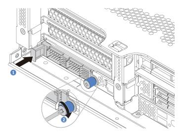
Figure 208. OCP 3.0 Ethernet adapter installation
