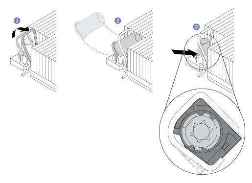
Figure 171. Installing a Torx T30 nut into the heat sink
