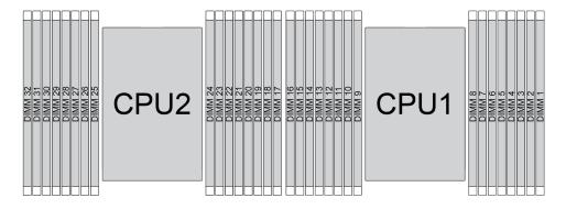
Figure 197. Memory module slots on the system board
