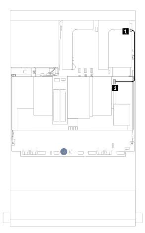
Figure 27. Cable routing for the super capacitor on the air baffle
