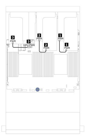
Figure 17. Cable routing for single-wide or double-wide GPU
