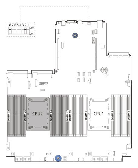
Figure 13. SW8 switch block on system board
