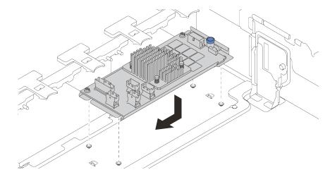
Figure 184. Internal CFF adapter installation
