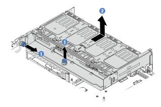
Figure 258. Removing the 8 x 2.5-inch rear drive cage
