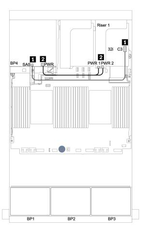
Figure 44. Cable routing for the rear 4 x 2.5 SAS/SATA backplane
