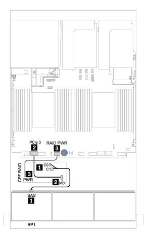
Figure 37. Cable routing for the 8 x 2.5-inch SAS/SATA configuration with one CFF 16i RAID/HBA adapter
