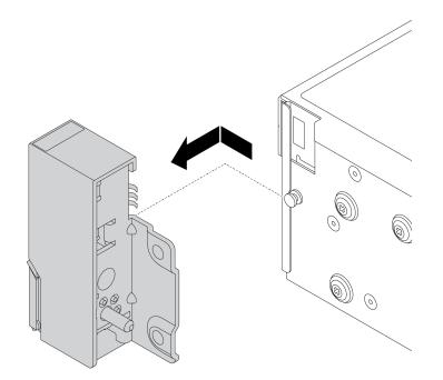
Figure 233. Rack latch removal
