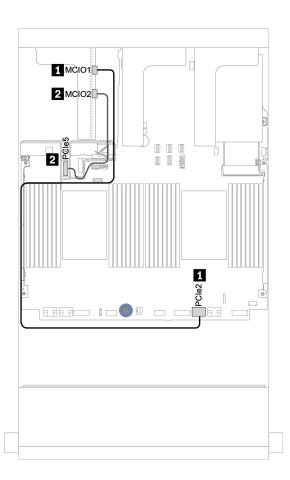
Figure 20. Cable routing for x8/x8 PCIe riser card 3 (configuration with 32 NVMe drives)
