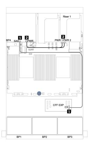
Figure 47. Cable routing for the 4 x 2.5-inch SAS/SATA rear backplane
