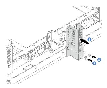
Figure 255. B1 rearwall bracket installation (middle)
