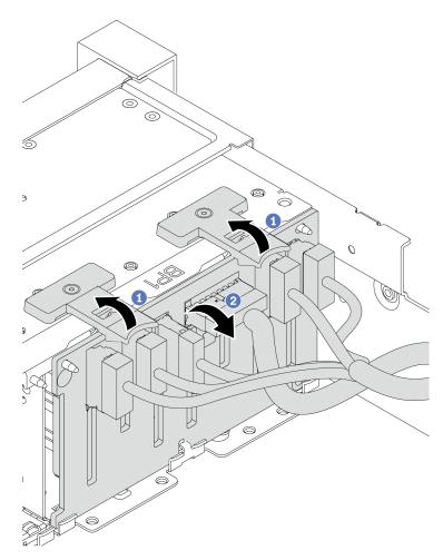
Figure 178. 2.5-inch drive backplane removal
