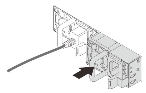
Figure 220. Hot-swap power supply installation
