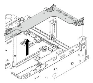
Figure 294. Removing the riser bracket
