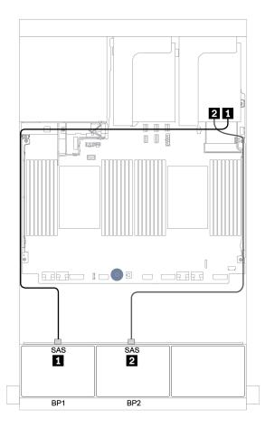
Figure 83. Cable routing for the 16 x 2.5-inch Anybay configuration with two Trimode 8i RAID adapters
