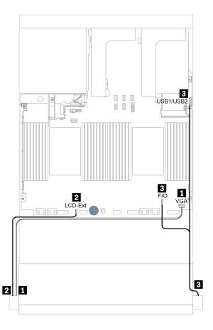
Figure 16. VGA connector and front I/O assembly cable routing
