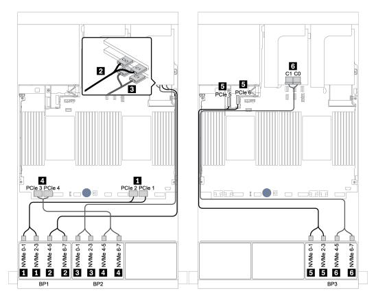
Figure 56. Cable routing for the 24 x 2.5-inch NVMe configuration with three retimer cards
