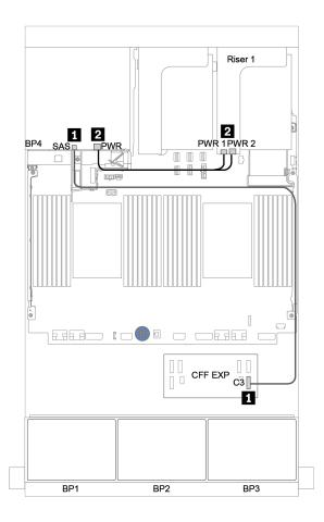
Figure 109. Cable routing for rear 4 x 2.5-inch SAS/SATA backplane
