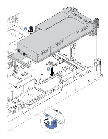
Figure 168. Installing the riser assembly
