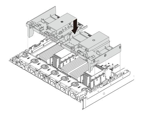
Figure 151. Installation of the standard air baffle
