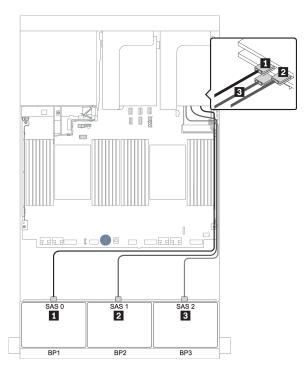
Figure 45. Cable routing for the 24 x 2.5-inch SAS/SATA configuration with one 16i HBA adapter and one 8i RAID adapter
