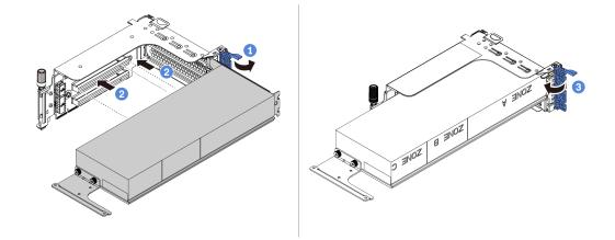
Figure 167. Installing the GPU adapter
