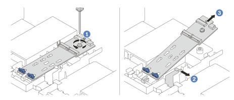
Figure 191. M.2 adapter removal
