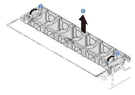
Figure 292. System fan cage removal
