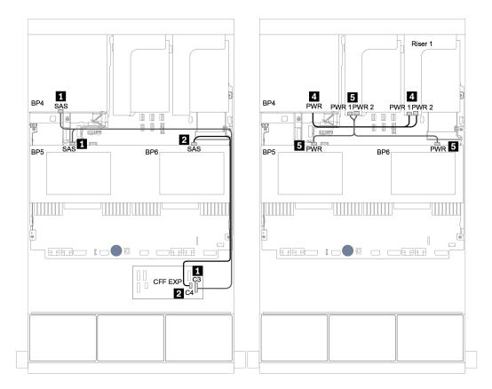
Figure 48. Cable routing for the two 4 x 2.5-inch SAS/SATA middle backplanes and one 4 x 2.5-inch SAS/SATA rear backplane
