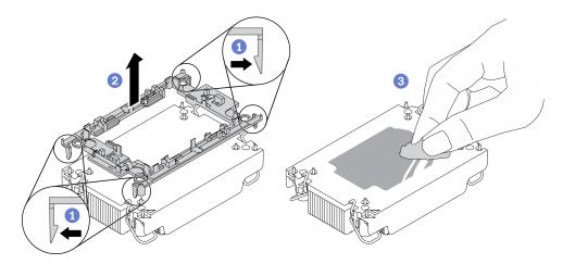
Figure 224. Separating a processor carrier the from heat sink
