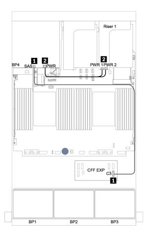
Figure 115. Cable routing for the rear 4 x 2.5-inch SAS/SATA backplane
