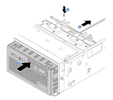
Figure 160. Front I/O assembly installation
