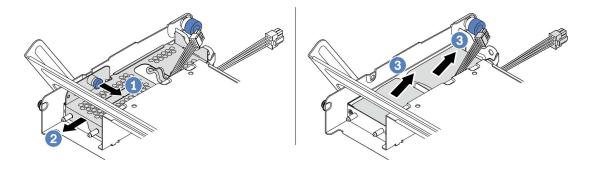
Figure 249. Removing the super capacitor module
