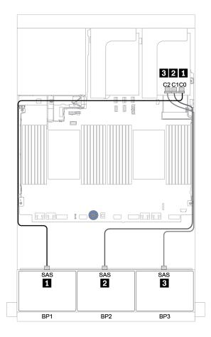
Figure 43. Cable routing for the 24 x 2.5-inch SAS/SATA configuration with one 32i RAID/HBA adapter
