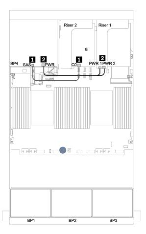
Figure 42. Cable routing for the rear 4 x 2.5-inch SAS/SATA backplane
