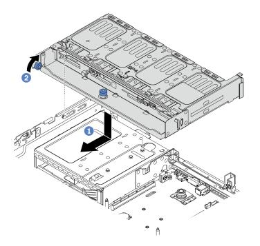
Figure 264. Installing the 8 x 2.5-inch rear drive cage
