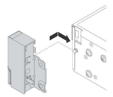
Figure 234. Rack latch installation
