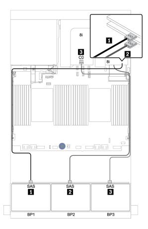
Figure 84. Cable routing for the 24 x 2.5-inch Anybay configuration with three Trimode 8i RAID adapters
