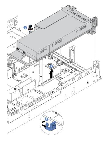
Figure 164. Removing the riser assembly
