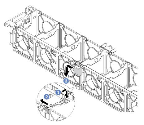
Figure 185. Intrusion switch removal
