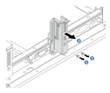
Figure 252. B1 rearwall bracket removal (middle)
