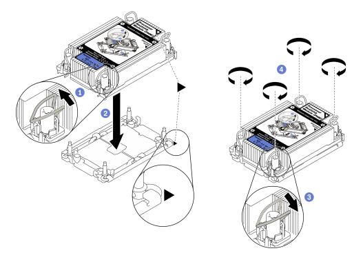
Figure 229. Installing a PHM
