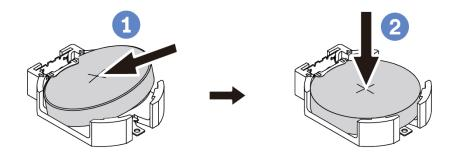
Figure 155. CMOS battery installation
