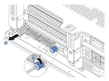
Figure 206. OCP 3.0 Ethernet adapter removal
