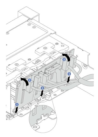
Figure 180. 2.5-inch drive backplane installation
