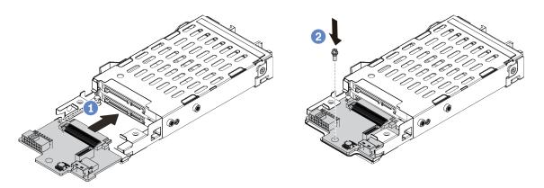
Figure 278. 7mm drive backplane installation (bottom)
