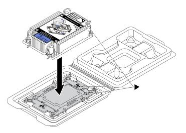
Figure 228. Assembling the PHM with processor in shipping tray
