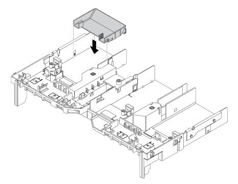
Figure 166. Installing the add-on air baffle
