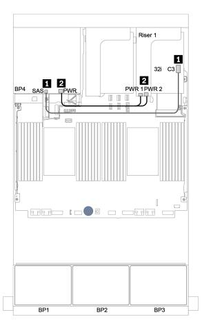
Figure 103. Cable routing for the rear 4 x 2.5-inch SAS/SATA backplane
