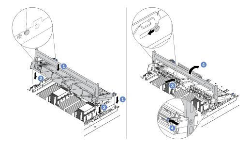
Figure 205. Installing the middle drive cage and drives
