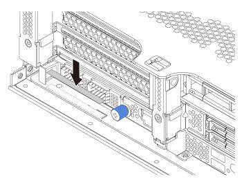
Figure 209. Attaching the OCP label
