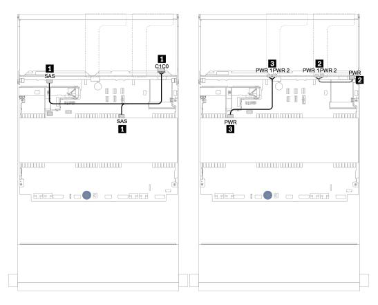
Figure 132. Cable routing for the 4 x 3.5-inch SAS/SATA middle backplane and 4 x 3.5-inch SAS/SATA rear backplane
