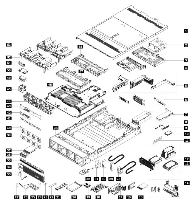
Figure 15. Server components (3.5-inch drive bay chassis)
