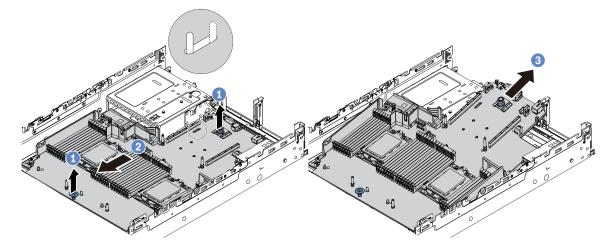
Figure 288. System board removal
