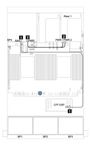
Figure 106. Cable routing for rear 4 x 2.5-inch SAS/SATA backplane
