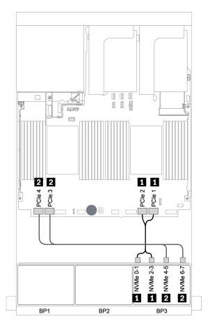
Figure 99. NVMe cable routing (two processors)
