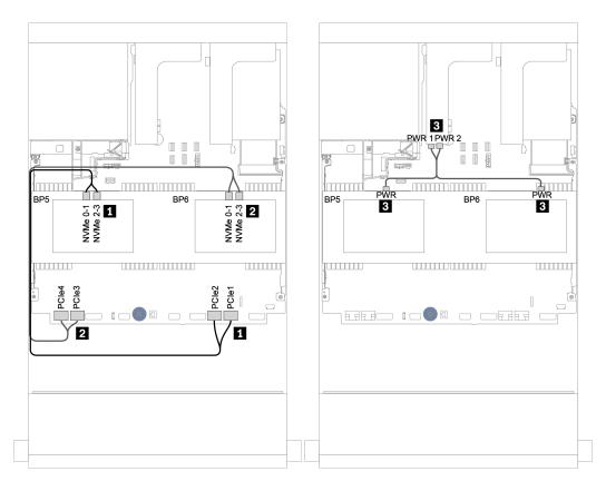
Figure 135. Cable routing for the two 4 x 2.5-inch NVMe middle drive backplanes
