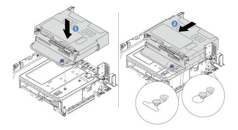
Figure 263. Installing the 4 x 2.5-inch rear drive cage
