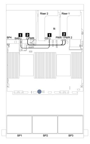
Figure 100. Cable routing for the rear 2.5-inch SAS/SATA backplane
