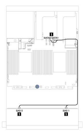
Figure 118. Cable routing for the 8 x 3.5-inch SAS/SATA configuration with onboard connectors
