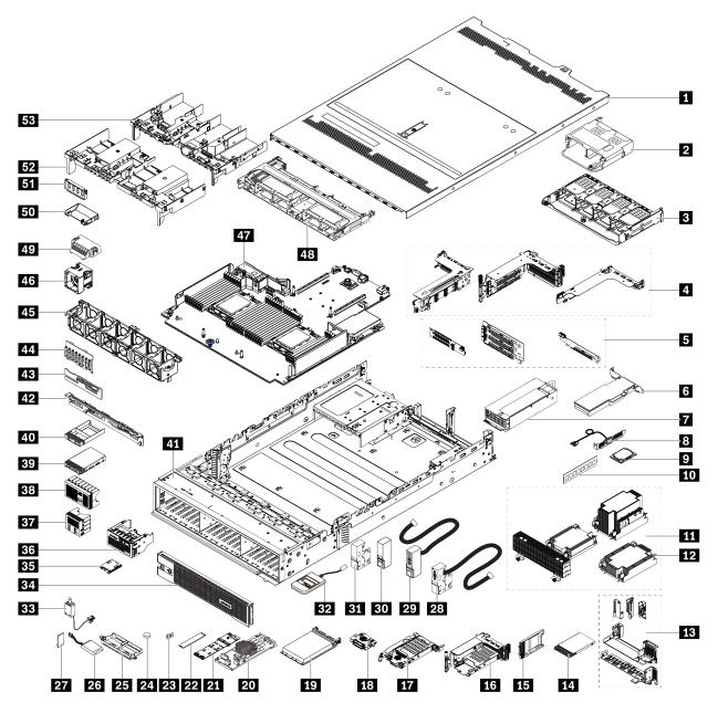
Figure 14. Server components (2.5-inch drive bay chassis)
