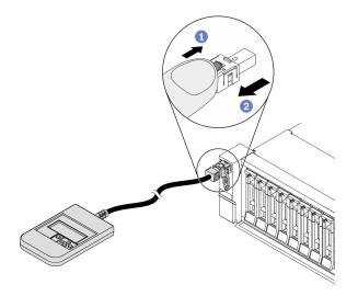
Step 1. Press the plastic clip on the plug in the shown direction.
