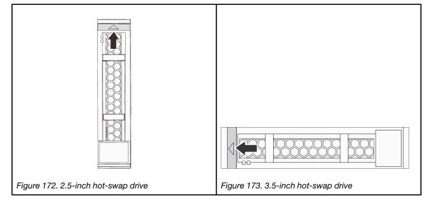
Step 3. Grasp the handle and slide the drive out of the drive bay.
