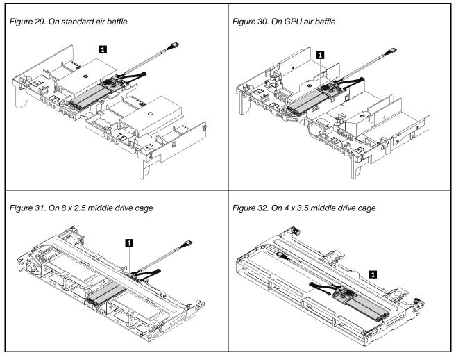
The following illustration shows the cable connection for M.2 module on the air baffle. It is the same for the M.2 module on other locations.
