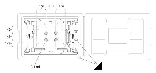
Figure 227. Thermal grease application with processor in shipping tray
