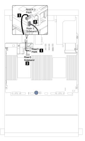
Figure 18. Riser card 3 power and sideband connection
