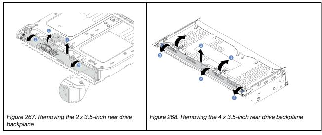
Step 1. Open the release latches in the direction as shown.
