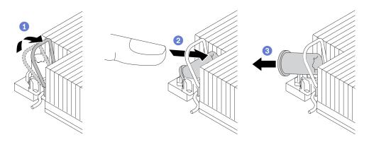
Figure 170. Removing a Torx T30 nut from the heat sink
