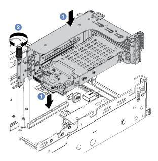
Figure 282. Riser assembly removal
