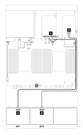
Figure 38. Cable routing for the 16 x 2.5-inch SAS/SATA configuration with one 8i RAID adapter
