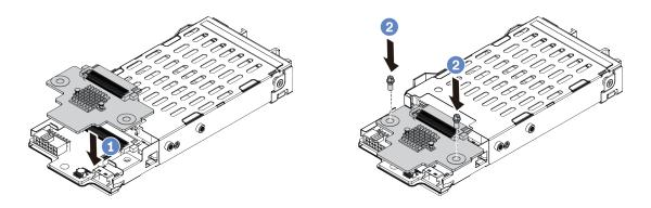
Figure 279. 7mm drive backplane installation (top)
