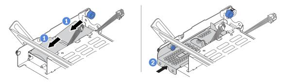
Figure 250. Installing the super capacitor module
