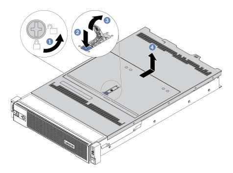
Figure 300. Top cover removal
