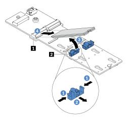
Figure 190. M.2 drive removal
