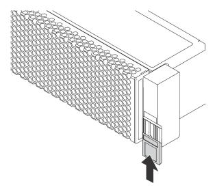
Figure 237. ID label plate installation
