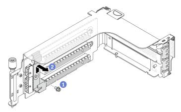
Figure 275. 7mm drive cage securing clip removal
