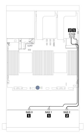
Figure 134. Cable routing for the 12 x 3.5-inch SAS/SATA configuration with one 16i RAID/HBA adapter
