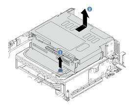
Figure 257. Removing the 4 x 2.5-inch rear drive cage
