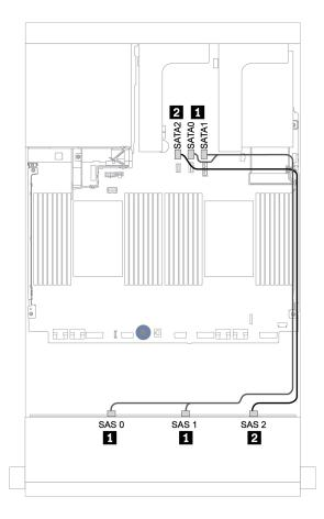
Figure 120. Cable routing for the 12 x 3.5-inch SAS/SATA configuration with onboard connectors
