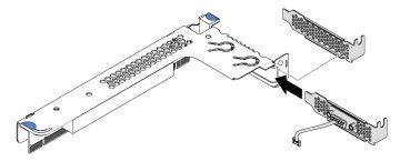
Figure 298. Installing the serial port module
