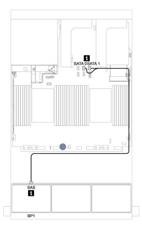
Figure 35. Cable routing for the 8 x 2.5-inch SAS/SATA configuration with onboard connectors
