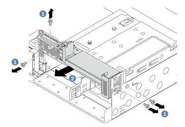
Figure 253. C1 rearwall bracket removal (right)
