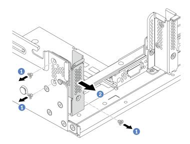
Figure 251. A1 rearwall bracket removal (left)
