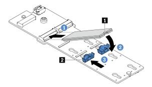
Figure 195. M.2 drive installation
