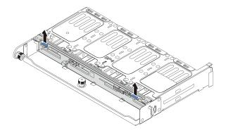
Figure 260. Removing the rear 8 x 2.5-inch drive backplane
