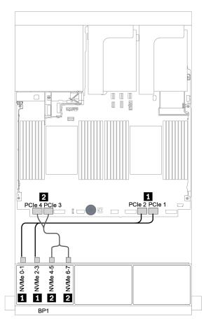
Figure 53. Cable routing for the 8 x 2.5-inch NVMe configuration with onboard connectors
