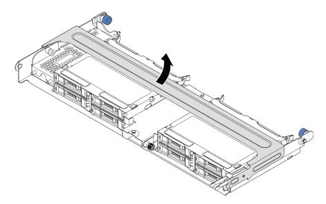
Figure 248. Opening the handle of the middle drive cage
