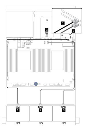
Figure 96. Cable routing for the 8 x 2.5-inch SAS/SATA + 16 x 2.5-inch Anybay configuration with one 8i/16i RAID/HBA adapter and two Trimode 8i RAID adapters
