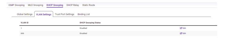
Users can click **Edit** button to enable DHCP snooping on a specific VLAN.
