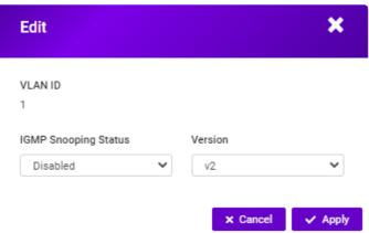
If Fast Leave is not used, a multicast querier will send a GS-query message when an IGMPv2/v3 group leave message is received. The querier stops forwarding traffic for that group only if no host replies to the query within the specified timeout period. If Fast Leave is enabled, the switch assumes that only one host is connected to the port. Therefore, Fast Leave should only be enabled on a port if it is connected to only one IGMP-enabled device.
