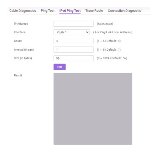
You can vary the test parameters by entering the data in the appropriate boxes. To verify accuracy of the test, it is recommended that you run multiple tests in case of a test fault or user error.
