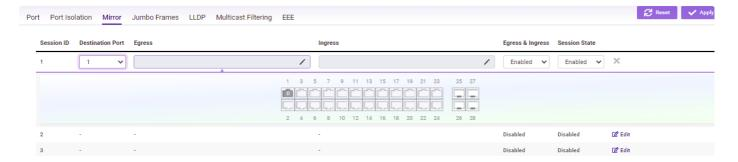
Mirror settings mirror network traffic by forwarding copies of incoming and outgoing packets from specific ports to a monitoring port. The packet that is copied to the monitoring port will be the same format as the original packet.
