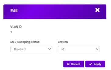
Select from the drop-down list whether to enable or disable MLD Snooping. Next, select to enable or disable Fast Leave for the specified VLAN ID.
