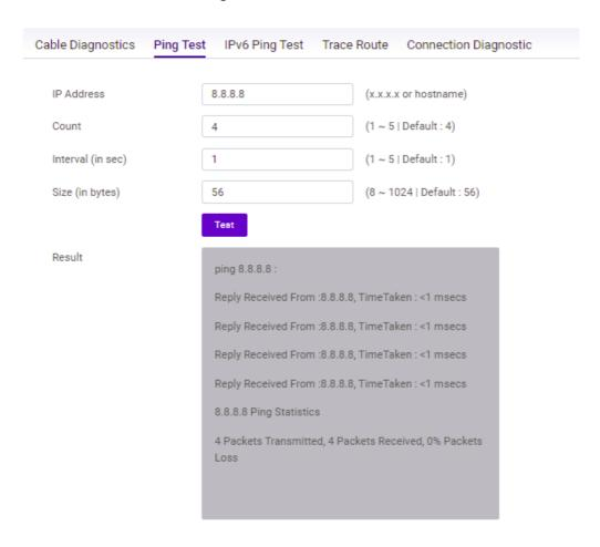
You can vary the test parameters by entering the data in the appropriate boxes. To verify accuracy of the test, it is recommended that you run multiple tests in case of a test fault or user error.
