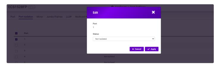
Port Isolation feature provides L2 isolation between ports within the same broadcast domain. When enabled, Isolated ports can forward traffic to **Not Isolated ports**, but not to other **Isolated ports**. **Not Isolated ports** can send traffic to any port whether **Isolated or Not Isolated**. The default setting is Not Isolated.
