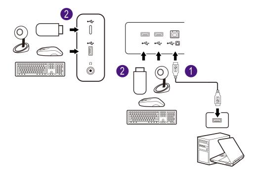
The USB-C™ port on the left or right side works as downstream port and connects with USB devices.
