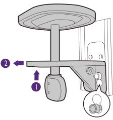
3. Release the screws completely so you can tighten them to the other set of screw holes.
