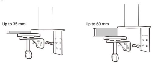
1. Use the provided Hex Key to half-release the screws that fix the C-clamp.
