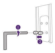
4. Half-fix the screws to the other set of screw holes.
