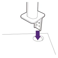
c. Attach the C-clamp to the stand and tighten the screws as instructed from step 5 to step 6 in Check desk thickness. on page 28.
