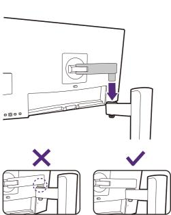
Raise the thumbscrew lid and tighten the thumbscrew as illustrated. Then push the lid back. If the upper arm is attached properly in the previous step, you will be able to tighten the thumbscrew.
