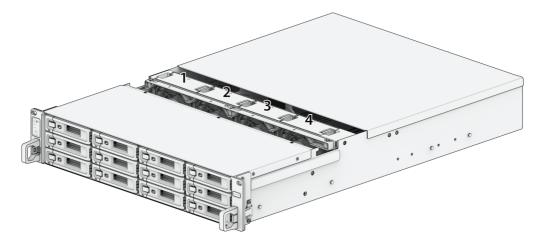
4. Find the malfunctioning fan. Lift up the fan to remove it.
