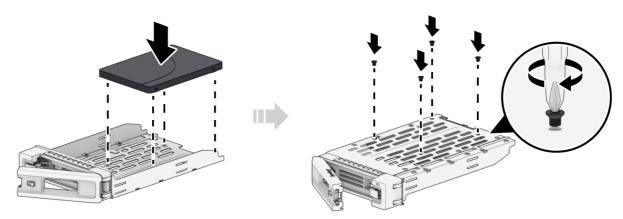
4. For 3.5" drives: Place the drive in the drive tray. Turn the tray upside down and tighten the screws to secure the drive in place.
