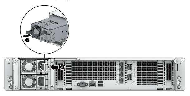
3. Prepare a new PSU. Insert it into the empty slot until you hear a click.
