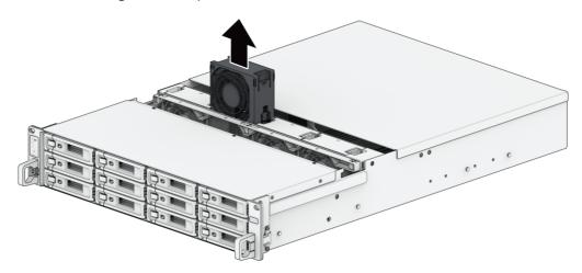
5. Prepare a new fan and slide it into the Synology NAS. Make sure that the fan is aligned properly.
