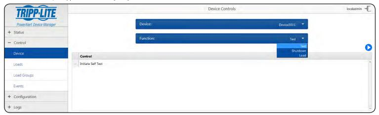
Figure 3-8: Individual Device Controls
