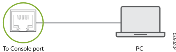
Figure 34: Connecting the ACX7100-48L Router Directly to a Management Console
