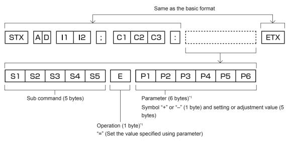
\*1 When transmitting a command which does not need a parameter, an operation (E) and parameter are not necessary.
