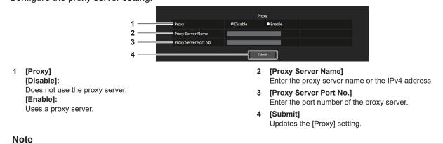
• [Proxy Server Name] does not support the IPv6 addresses.
