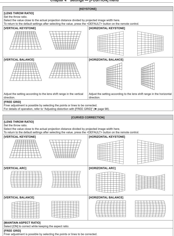
For details of operation, refer to "Adjusting distortion with [FREE GRID]" (→ page 98).
