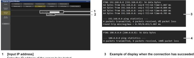
Enter the IP address of the server to be tested.
