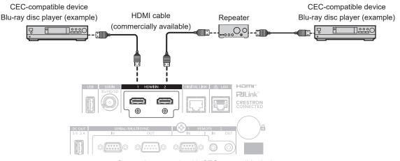
Connection example with CEC-compatible device
