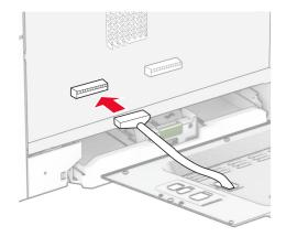
**9** Connect the fax interface cable to the controller board.
