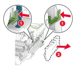
**Note:** To avoid spilling the toner, place the bottle in an upright position.
