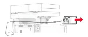
**6** Remove the used power supply.
