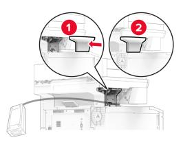
**Note:** Secure the power supply properly.
