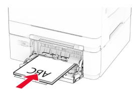
• Load envelopes with the flap side up and against the right side of the paper guide.
