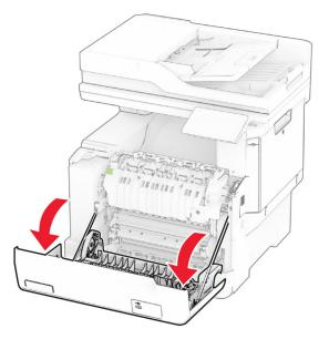
${\bf 2}~$  Open the fuser access door, and then remove the jammed paper.
