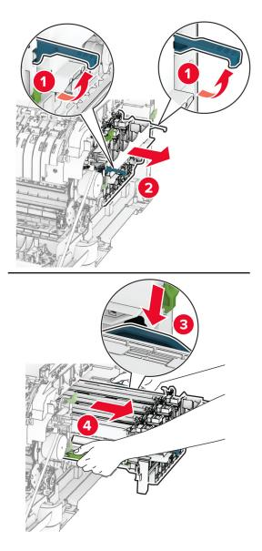
7 Remove the used developer unit.
