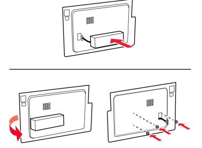
8 Connect the hard disk interface cable to the controller board.
