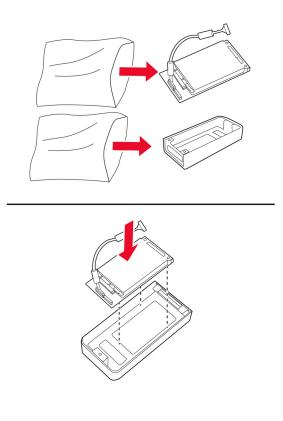
**7** Attach the hard disk to the controller board shield.
