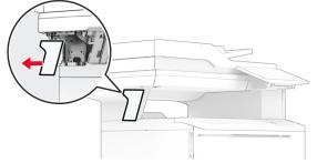
5 Insert the power supply through the printer, and then connect it to the convenience stapler.Note: To avoid damaging the convenience stapler, use only the power supply that came with it.
