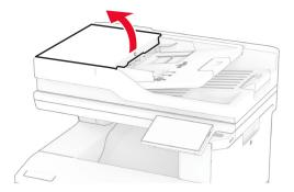
**2** Remove the used ADF pick roller.
