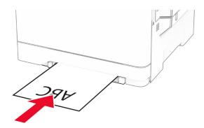
• Load envelope with the flap side up and against the right side of the paper guide.
