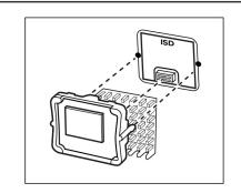
**7** Attach the controller board shield, and then install the screws.
