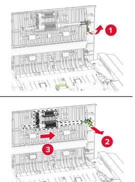
**3** Remove the used ADF separator roller.
