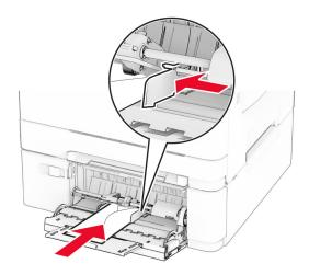
**Warning—Potential Damage:** Do not use envelopes with stamps, clasps, snaps, windows, coated linings, or self-stick adhesives.
