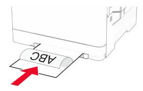
• For two-sided printing, load letterhead with the printable side faceup and the top edge entering the printer last.
