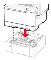
**Note:** To avoid invalid configuration, when installing both the 550-sheet tray and 650-sheet tray, always place the 550-sheet tray below the 650-sheet tray.
