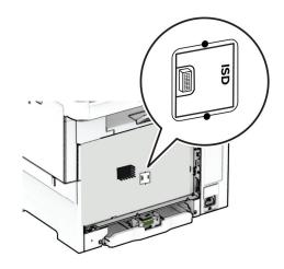
**6** Insert the storage drive to the ISD connector.
