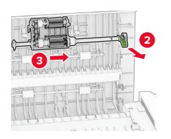
**3** Remove the ADF separator roller.
