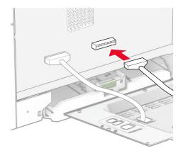
**10** Attach the controller board shield, and then install the screws.
