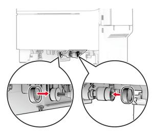
Note: Make sure that the edges of the pick tire treads are facing downward.
