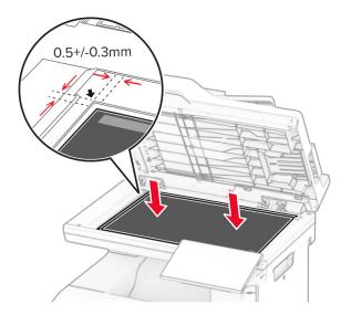
**5** Close the scanner cover to attach the new scanner glass pad.
