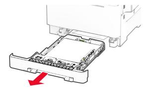
**Warning—Potential Damage:** A sensor inside the optional tray is easily damaged by static electricity. Touch a metal surface before removing the jammed paper in the tray.
