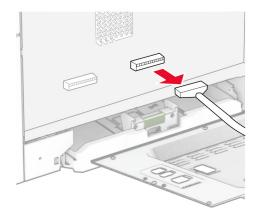
**5** Remove the hard disk port cover from the controller board shield.
