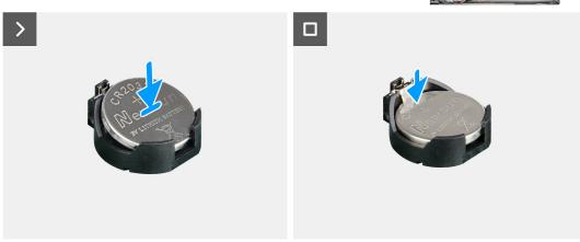
With the positive side (+) facing up, insert the coin-cell battery into the battery socket on the system board and snap the battery into place.
