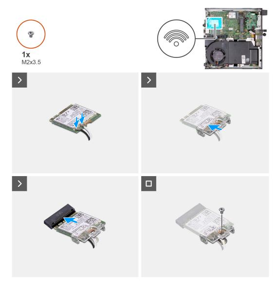
1. Connect the antenna cables to the wireless card.
