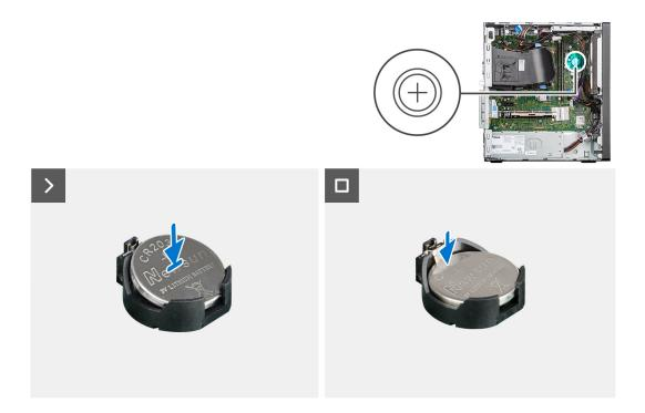
Insert the coin-cell battery into the socket with the positive side (+) label facing up and snap the battery in the socket.
