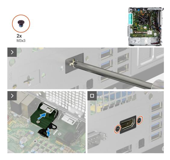
1. To remove the dummy metal bracket, insert a star-head screwdriver in the hole of the bracket, push the bracket to release the bracket, and then lift the bracket out from the system.
