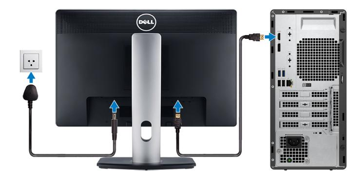
() **NOTE:** If you ordered your computer with a discrete graphics card, the HDMI and the display ports on the back panel of your computer are covered. Connect the display to the port on the discrete graphics card.
