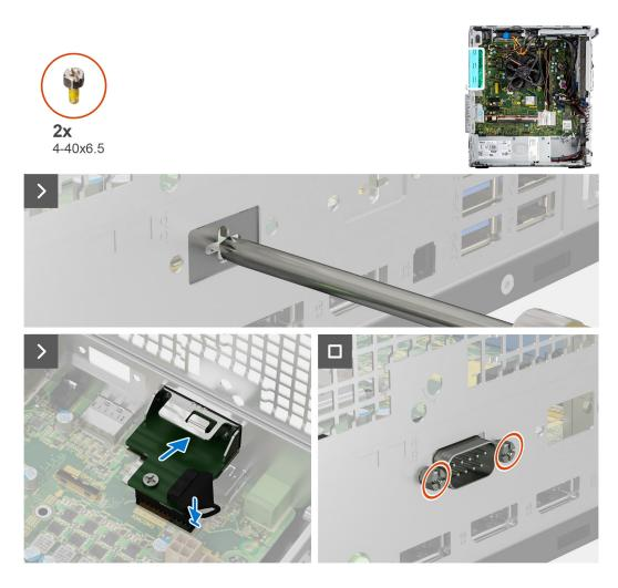
1. Using a screwdriver, remove the serial module cover from the chassis.
