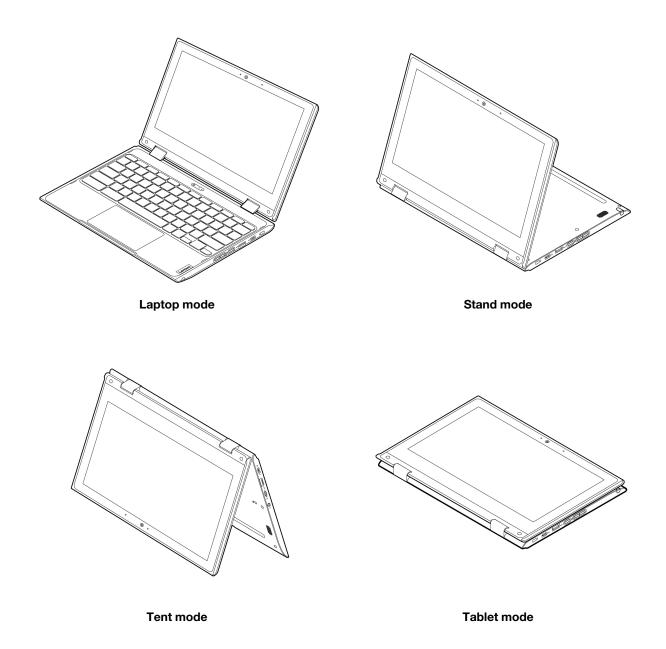
**Warning**: When operating in the tablet mode with any external device connected, the upper case (keyboard's side) of the Chromebook may become hot. Avoid keeping your hands, lap, or any part of the body in contact with the upper case for over one minute.
