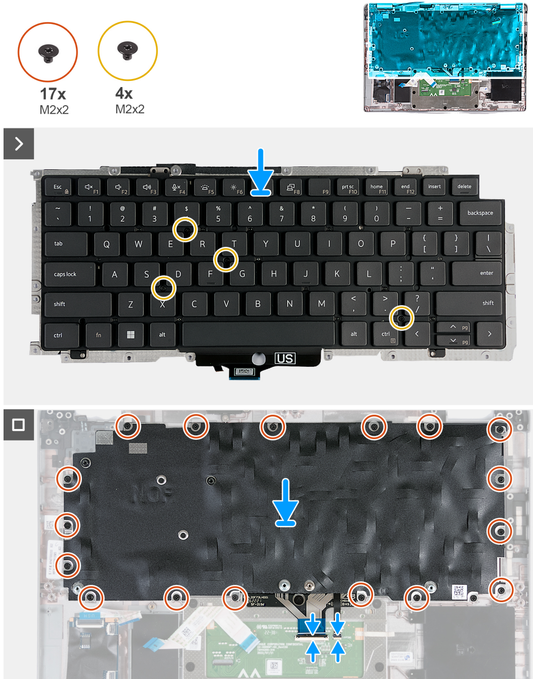
Figure 62. Installing the keyboard
