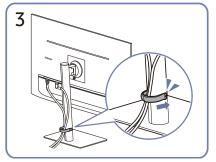
Put both cables in the cable holder on the stand (HOLDER-STAND CABLE) to organize the cables, as shown in the figure.
