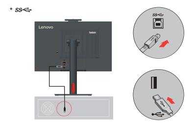
Connect one end of the USB cable to the USB downstream terminal on the side of the
