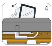
4D. Once the iPad is inside, plug the lighning charging cable into the power socket. Then place the internal front (hard) cover on the top of the case and gently clip all four sides shut.
