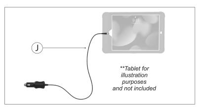
6A. Plug one end of your car power adapter (J) into the dock (I) charging port. Plug the other end into your vehicle auxiliary power outlet.
