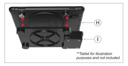
7A. Align the battery pack (H) to the battery pad (I) on the right side by aligning the magnets, so the tablet charges properly.
