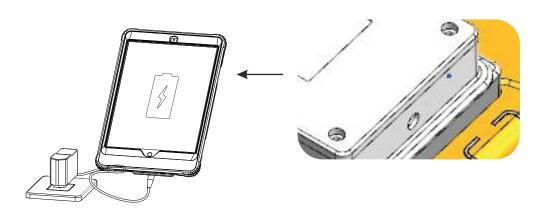
8A. Connect the AC/DC power supply to the charging plate as pictured.
