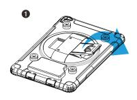
5A. Locate kickstand at case rear and fold out underneath strap.
