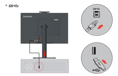
4. Connect one end of the USB cable to the USB downstream terminal on the side of the monitor, and connect the other end of the USB cable to an appropriate USB port on your device.
