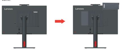
3. Pull the computer out of the computer bay. Then, pivot the cable cover as shown to the closed position.
