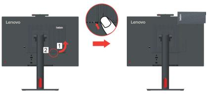
2. Pivot the rear Wi-Fi antenna downward at an angle of about 90°. Then, hold the thicker end of the rear Wi-Fi antenna and unscrew it from the computer.
