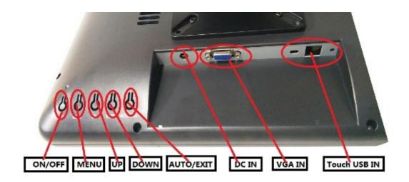
TOUCH USB: this is connected to PC's USB Ports; used for touch function
