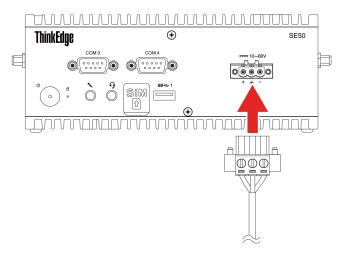
5. Reconnect the external cables to the corresponding connectors on the computer, and then reconnect the power cord to the electrical outlet.
