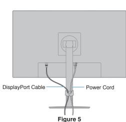
5. Connect the power cord to a power outlet.
