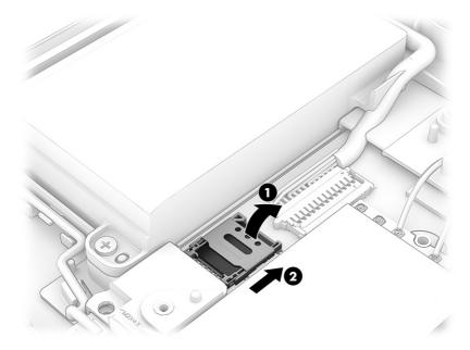
To remove the SIM card, reverse the procedures as described previously.
