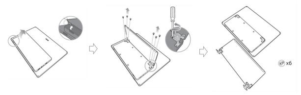
Note: If installing with a wall mounting kit, it is recommended to use VESA mounting kit (100mm  $\times$  100mm) with M4  $\times$  10 (L) mm screws to fix your monitor on the wall.
