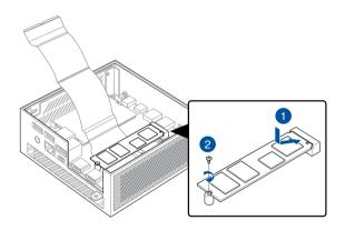
3. Before replacing the bottom cover, ensure to remove the plastic film on the thermal pad.
