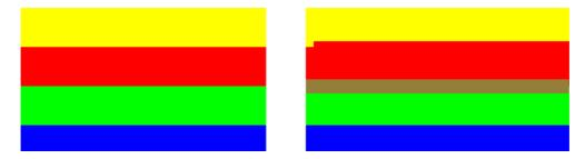
Finally, a special pattern for checking the printer's printhead alignment can be found at the top left of the diagnostic sheet. This pattern has no number as it is not used for scanner checking. It is made of three colored crosses that may be used to identify the problem in question. The correct pattern is shown on the left, an example of misalignment on the right.
