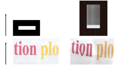
Open and close the scanner lid by pushing it down until you hear a click. Then repeat your scan and visually check that the original advances correctly through the scanner path. If not, call HP support and report an "incorrect paper advance" error. Remember that your scanner is not intended to work with originals thicker than 0.75 mm (29 mil).
