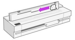
5. For more thorough cleaning, clean the calibration surfaces and the feed rollers.
