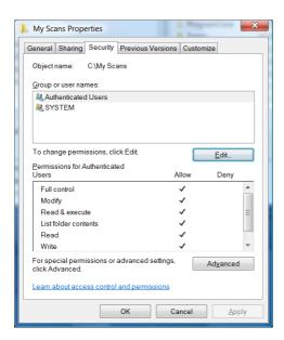
The 'scanner user' can now access the folder and write files to it. Next, you must configure the printer to send scans to the folder.
