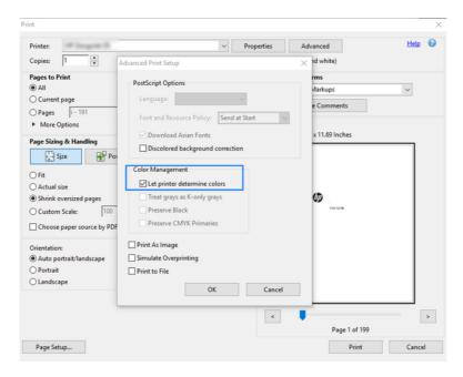
5. If the document contains several color profiles and you are not sure what the result will be, you can flatten the document first and print it as seen on the screen. To do this, check the box Print As Image in the Advanced Print Setup dialog box. In this case, the rasterization is performed by
