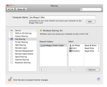
The 'scanner user' can now access the folder and write files to it. Next, you must configure the printer to send scans to the folder.
