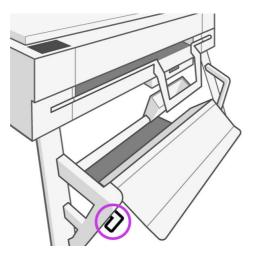
4. Hold down one end of the bottom to prevent it from rotating before lifting the front board into the up position. This completes the regular bin style configuration.
