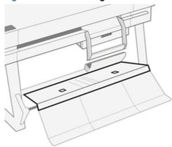
• For A0/E size portrait size collection: From the default configuration, standing in front of the printer, pull the backboard forward using the two square finger grooves. The backboard will rotate downwards and reveal a deeper media fabric path for A0 roll size collection.
