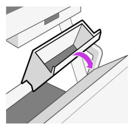
3. Check to see if the transfer is correctly done, the bottom pole should be visible and free to rotate upwards.
