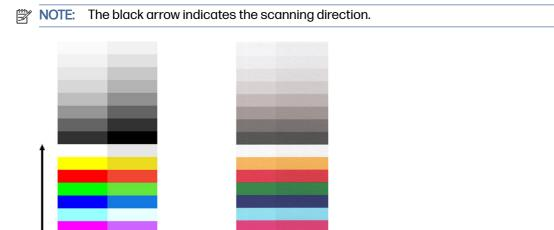
Sometimes the color mismatch between adjacent modules can be enormous, showing a serious scanner malfunction, as in the following example. If this occurs, see <u>Completely wrong colors on page</u> 139.
