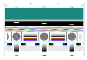
Some of the most common defects that may appear in a printed diagnostic plot are described below. If you find any of these problems, you should follow the recommended recovery procedure. See the Troubleshooting print-quality issues on page 114. Once the printer has been diagnosed and it is working correctly, you can reprint the diagnostic sheet as described in <u>Prepare the printer and the paper to print</u> the diagnostic sheet on page 143.
