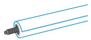
6. Looking from the front of the printer, put the blue paper stop on to the open end (left side) of the spindle, and push into the end of the roll.
