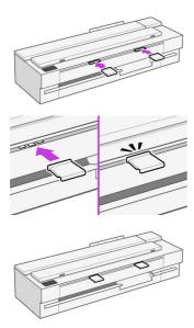
The refeed preventers are designed to prevent this situation from occurring. Make sure that they are always installed.
