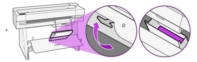
For A4 and ANSI A size cut-sheet collection: The length adjuster needs to be in the down position
