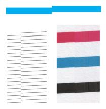
The four vertical thin black lines at the beginning and the end of the diagnostic plot show, approximately, the position of the intersection between scanbars, where this kind of error usually appears. If the error appears outside these areas, call HP support and report "line discontinuities within a scanbar".
