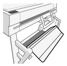
2. Lift and transfer the stacker to the lower slot position, ensure only the top pole is inserted onto the lower of the left and right semi circular slots.
