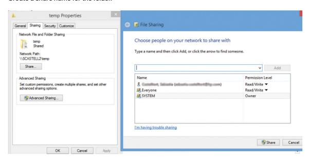
Once the shared folder is created, go to the Embedded Web Server and follow the instructions under the Scan to network folder setup process.
