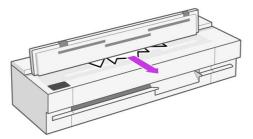
Or pull it from the front bottom area between the scanner platen and front window.
