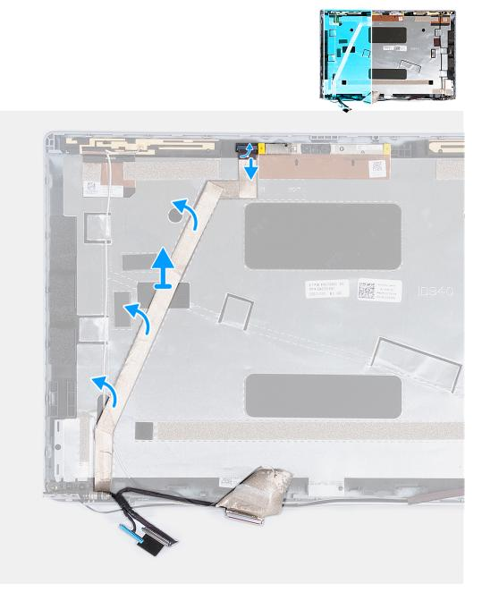
Figure 49. Removing the display cable
