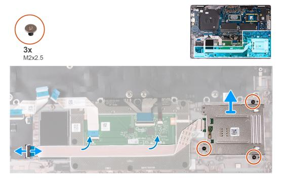
Figure 57. Removing the smart card reader
