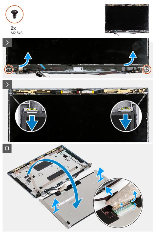
Figure 43. Removing the display panel
