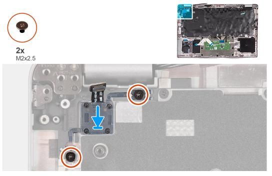
Figure 60. Installing the power-button board
