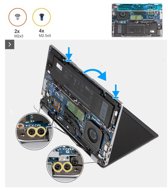
Figure 39. Installing the display assembly - For computers shipped with 5G card
