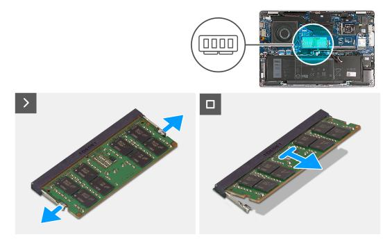
Figure 6. Removing the memory module
