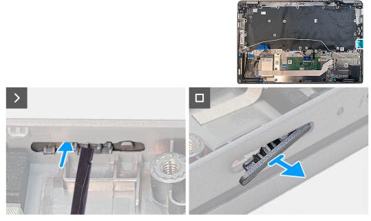
Figure 65. Removing the dummy SIM-card slot filler
