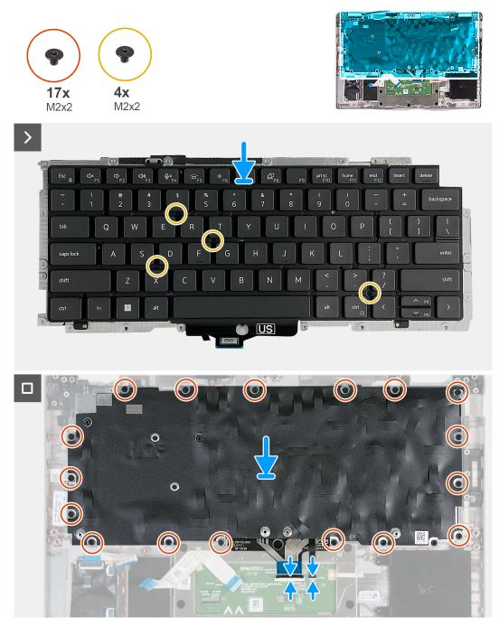
Figure 62. Installing the keyboard
