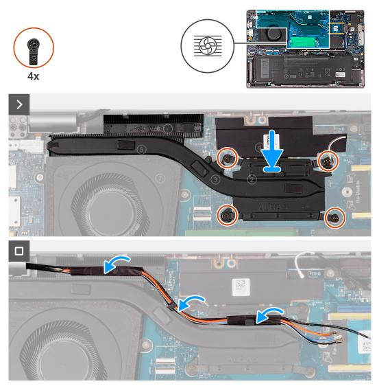
Figure 26. Installing the heat sink - For computers shipped with 5G card
