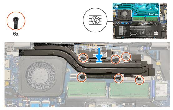
Figure 28. Installing the heat sink
