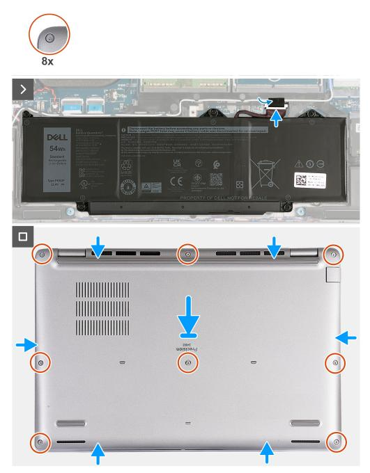
Figure 5. Installing the base cover
