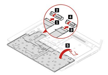
2. Insert the keyboard into the keyboard bezel as shown. Ensure that the top edge of the keyboard (the edge that is close to the display) is under the keyboard bezel.
