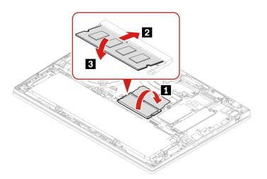
**Note:** For ThinkPad T14 Gen 4 Intel models, memory module replacement might cause memory retraining. For details, see "Detect memory retraining (for Intel models only)" on page 32.
