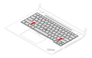
3. Pivot the keyboard slightly upward **I** and then turn over the keyboard **2**.
