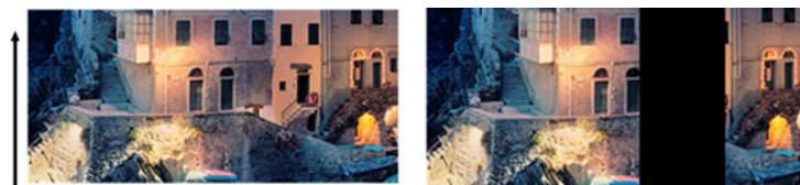
Original Scan affected by a failing scanbar
